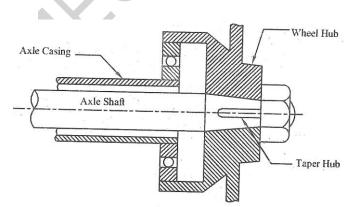
So, heavier loads may be carried without danger of axle breakage. In this case the inner end of the axle shaft is in the differential. Thus 75 % of the vehicle's weight goes directly from the axle housing to the wheel. The axle is keyed rigidly to the hub.
