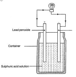
*Simple cell* The lead acid battery is mostly used in automobiles. The principle employed in this case is as follows: There are two rods; one is of pure lead and other rod is of pure lead peroxide which are in a solution of dilute sulphuric acid as shown in the fig. Then an electric voltage is generated between the rods, the lead peroxide forms the positive pole and pure lead forms the negative pole.
