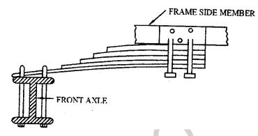
• This system also called cantilever spring system was mainly used in cars in olden days both at front and rear end (crosley car). In this case half-elliptical spring is mounted in inverted position with its heavy end bolted to the chassis frame.
