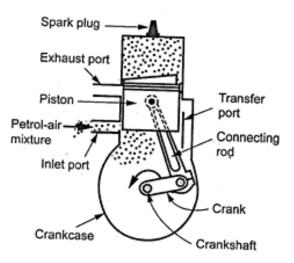
The crown of the piston (i.e., top of the piston) is shaped in such a way to assist in deflecting the fresh charge upwards in the cylinder and help scavenging.
