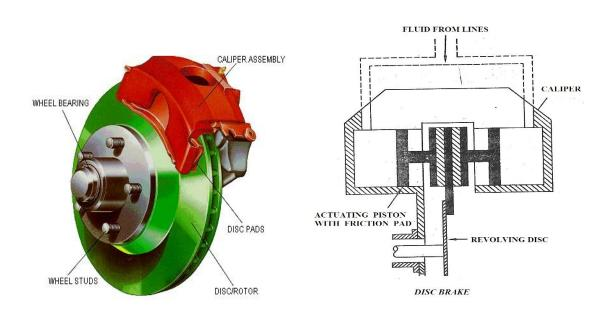
• When the brake pedal is applied the fluid will be displaced from the master cylinder to the wheel cylinder pistons. This will exert equal and opposite pressure on the friction pads by forcing them against the rotating disc to grip it.
