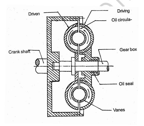
The oil is thrown out against the curved interior surface because of a centrifugal force. Then, it is directed across, to the runner and returned to the impeller. When the efficiency of the coupling is highest, under best operating conditions, runner speed is almost equal to the impeller. The lagging of the driven unit behind the driver unit is known as slip.
