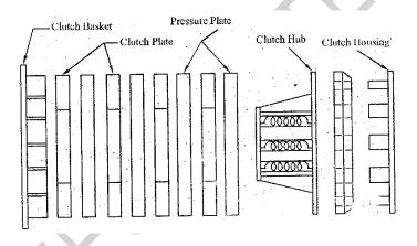
It consists of four clutch disks, four pressure plates, clutch hub and springs. When the control lever is operated the clutch gets disengaged. Then the plates will not press on the clutch disks. There is no power transmission taking place when the clutch lever is released, the springs press the pressure plates as well as clutch plates, and it transmits the power from engine.
