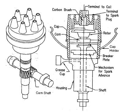
The H.T cables lead the high voltage to the spark plug. The central terminal is connected to the secondary of the ignition coil. As the distributor spindle has to rotate at half the crank shaft speed, the drive for it is taken from the cam shaft through spiral gears. As the distributor spindle rotates, the rotor point comes into contact with each terminal in the cap. Thus the high voltage passes to each cylinder in turn. Fig. shows the exploded view of distributor.
