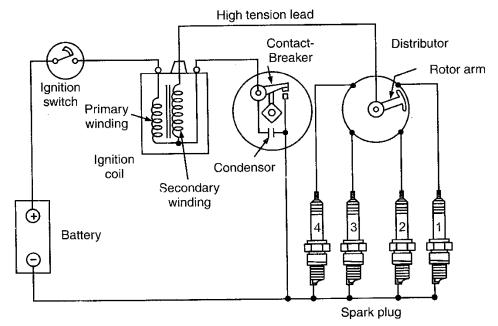
Battery ignition system for four-cylinder engine
