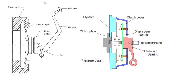
It consists of the foot pedal, Fork lever, Fork, thrust bearing and fingers as shown in fig. The release bearing is held in a fork and is free to move over the clutch shaft. The fork in turn is connected with the foot pedal through the fork lever. The thrust bearing operates the clutch release fingers provided in the pressure plate.
