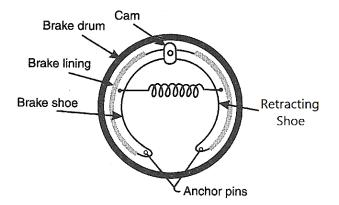
Mechanical Brakes (Cam - Operated)
