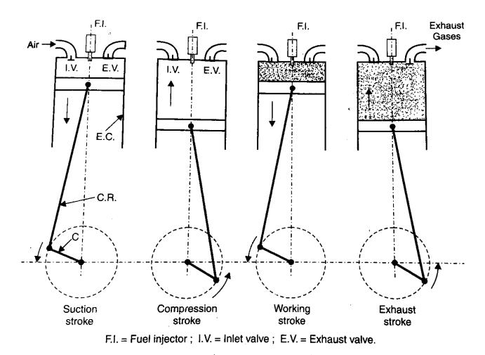
Four stroke Diesel cycle engine.
