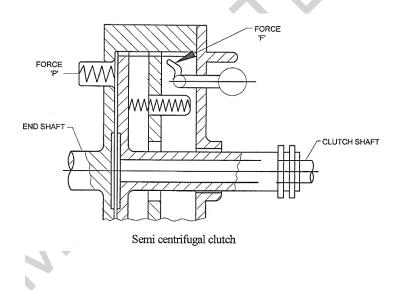
However at higher speeds, the weight C, due to the centrifugal force moves about A as fulcrum thereby pressing the pressure plate. The centrifugal force is proportional to the square of the speed so that adequate pressure level is attained. Fig. Shows the variation of force on the pressure plate at various speeds
