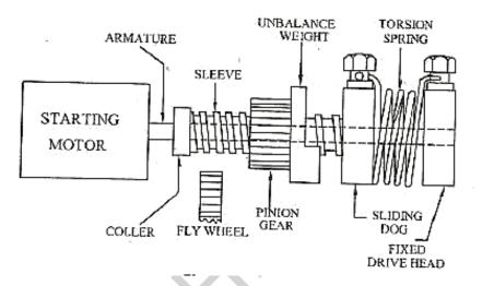
When the motor starts, the armature shaft rotates. Due to the unbalance weight, the pinion cannot rotate and it moves axially towards the motor. The pinion is engaged with flywheel. There is collar attached on the sleeve. Now the pinion is engaged and rotates the flywheel of the engine and the engine starts. When the engine starts, the self-starter switch is off.
