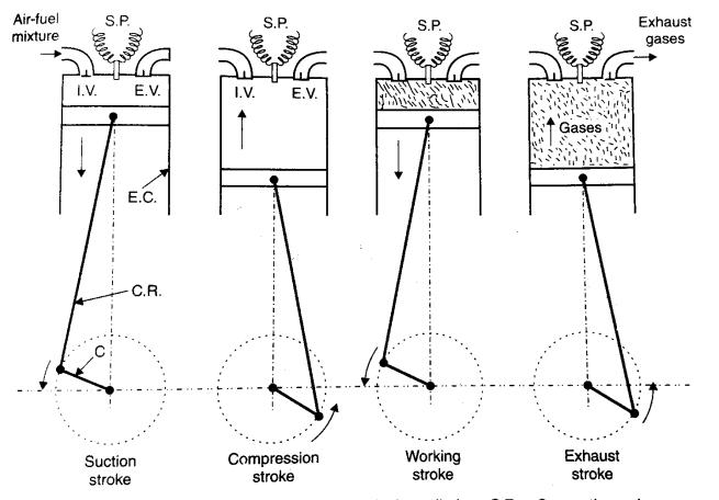
I.V. = Inlet valve ; E.V. = Exhaust valve ; E.C. = Engine cylinder ; C.R. = Connecting rod ; C = Crank ; S.P. = Spark-plug.
