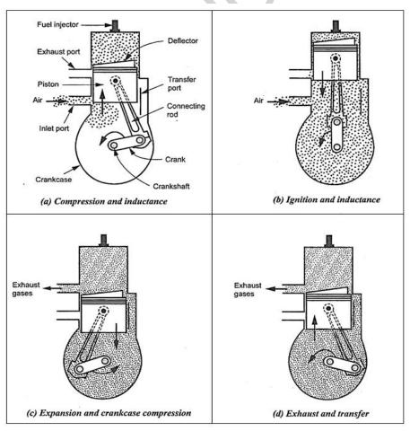
Two Stroke - Diesel Engine
