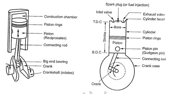
The main components of an IC engine and their functions are presented below
