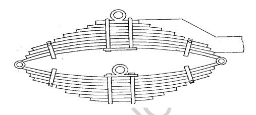
Full elliptical spring consist of two semi-elliptical springs joined together oppositely. This type of spring was used in old cars. They do not maintain correct axle alignment.
