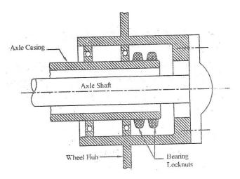
The axle shaft is not supported by bearings but it is positioned at its ends. Hence, in this method, the axle is relieved of all strains due to the load of the vehicle or end thrust. Being free from all other strains, its duty is only to transmit a rotary motion to the wheel. Without disturbing the axle hub and the wheel, the axle shaft can be removed from the casing.
