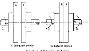
Principle of Friction Clutches.
