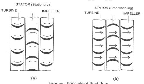
Figure : Principle of fluid flow
