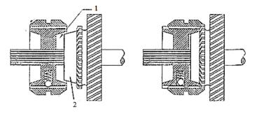
(a) Disengaged position (b) Engaged position
