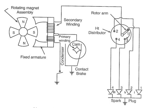
Magneto ignition system for a four cylinder engine
