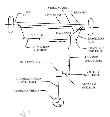
When the steering wheel is rotated the drop arm moves towards or away from the front wheel depending upon the direction of turn right or left
