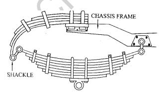
It is a combination of semi-elliptical and quarter elliptical spring. In the olden days it was popular but has been now replaced by semi-elliptical spring
