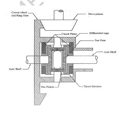
But it is provided with two sets of multi plate clutch as shown in the figure. Moreover, the ends of the pinion shafts are made to float usually in notches in the differential cage. The clutches are positioned between the sun gears and the differential cage. If at all there exists any difference between the speeds of the sun gears and the cage, it is limited by the frictional resistance between the clutches and sun gears. The driving torque is increased by this increased frictional resistance.
