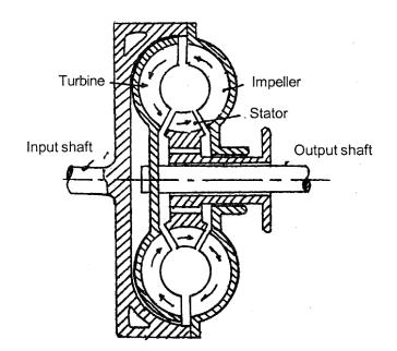
Fig. Torque converter
