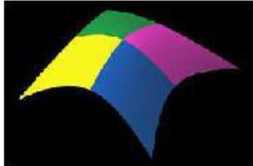
four parametric surface patches joined together to form a larger surface area
