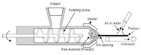
Fig. 4.18 Schematic extrusion moulding
