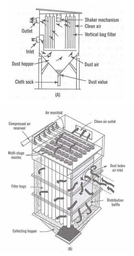
Fig. 5.7 (A) Bag filter (B) Schematic arrangement of an ultra-jet type filter
