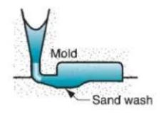
(4) Scab: It is caused by portions of the mould surface flaking off during solidification and gets embedded in the casting surface.
