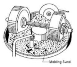
Fig. 1.26 Sand mixing muller
