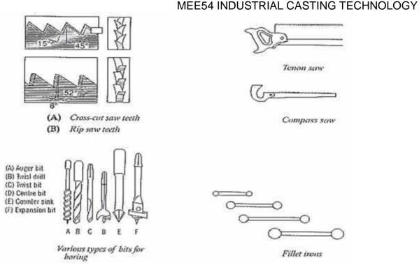
Fig 1.10 Hand Tools for Wood Patternmaking
