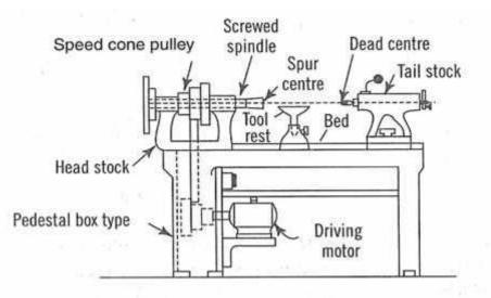
Fig 1.3 Woodworking lathe
