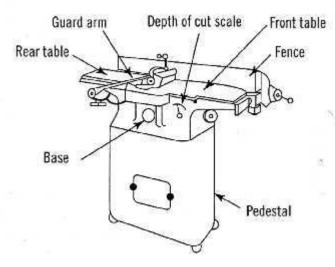
Fig 1.5 Wood Jointer
