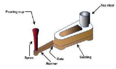
Fig 1.2 a typical pattern attached with gating and risering system
