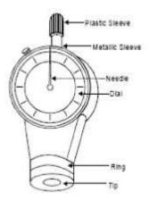
Fig. 1.25 Mould hardness tester
