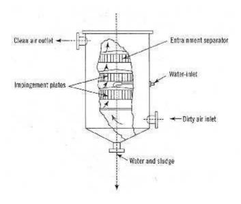
Fig. 5.9 Wet centrifugal dust collector
