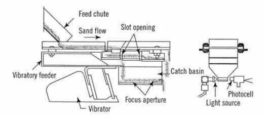
Fig. 5.15 Mouldability Controller
