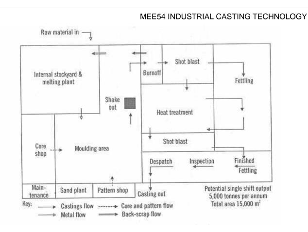
Fig. 5.12 Typical Layout of a grey iron foundry
