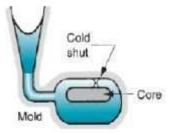
(3) *Cold shots*: forming of solid globules of metal that are entrapped in the casting. Proper pouring procedures and gating system designs can prevent this defect.
