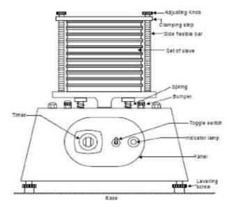
Fig. 1.22 Grain fitness testing mechanical shaker
