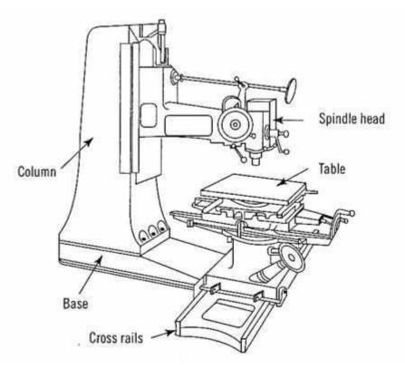
Fig 1.9 Block diagram of pattern milling machine
