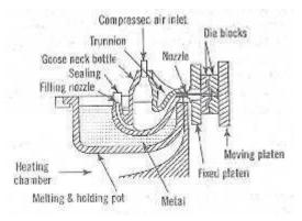
Fig. 4.5 Air-blow type die-casting machine
