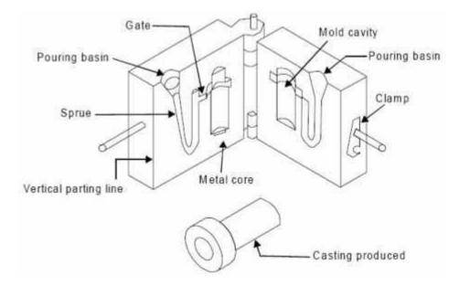
Fig. 4.1 A typical permanent mould
