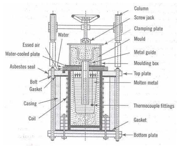
Fig. 4.6 Low-pressure die-casting machine
