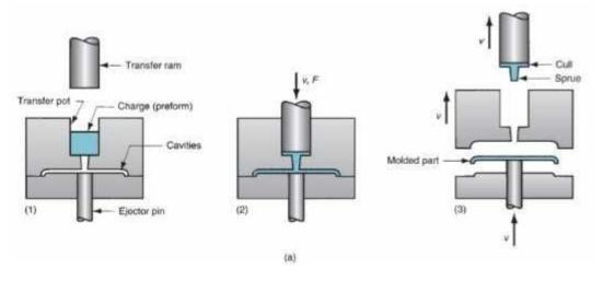
Fig. 4. 16 (a) Pot transfer moulding, and (b) plunger transfer moulding.
