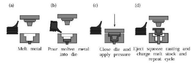
Sequence of operations in the squeeze-casting process.
