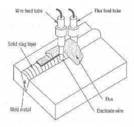
Fig. 5.1 Submerged Arc Welding
