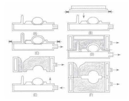
Fig. 4.14 Steps in vacuum moulding process
