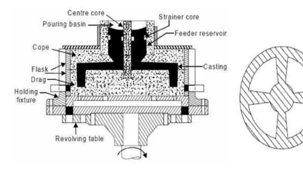
Fig. 4.9 Semi-centrifugal casting setup
