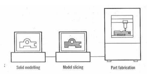
Fig 1.11 Main steps in rapid prototyping
