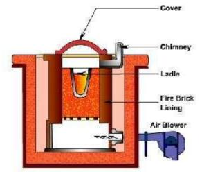
Coke Fired Crucible Furnace
