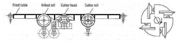
Fig 1.6 Principle parts of a wood Planer
