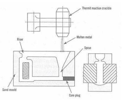
Fig. 5.2 Arrangement of thermit welding for casting repair
