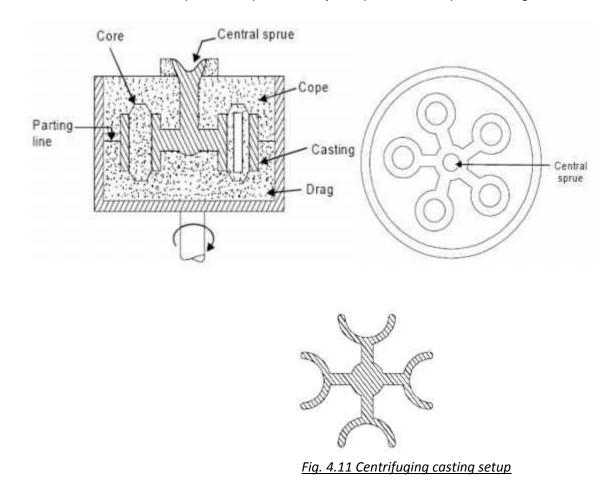
Fig. 4.12 Article produced by centrifuging casting process
