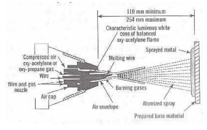
Fig. 5.3 Metal Spraying
