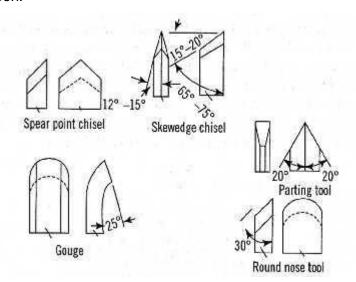
Fig 1.4 woodworking lathe tools
