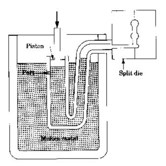
Fig. 4.2 Plunger type hot-chamber die-casting Machine
