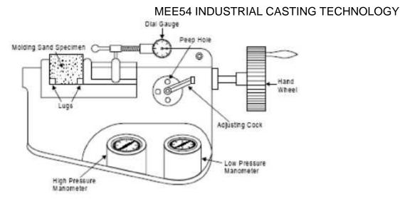
Fig. 1.23 Strength testing machine
