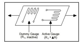
Figure 5. Use of Dummy Gage to Eliminate Temperature Effects
