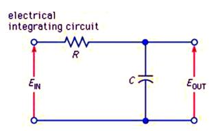
For time-varying input, if the resistance R shown in the schematic diagram is very large compared with the capacitive reactance  $X_C$  of the capacitor C, the current will be almost in phase with the input
