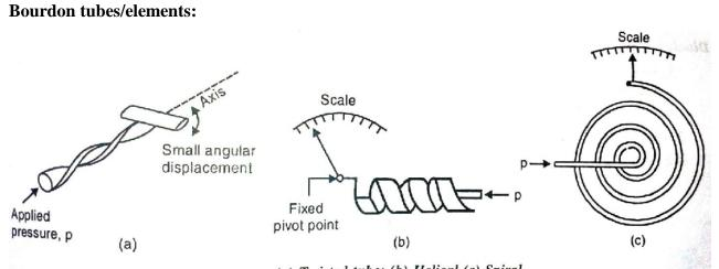
(a) Twisted tube; (b) Helical (c) Spiral.
