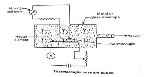
The heater element is supplied with a constant electric energy and its temperature is measured by a thermocouple. The voltage measuring instrument can be directly calibrated to read the pressure of the gas.
