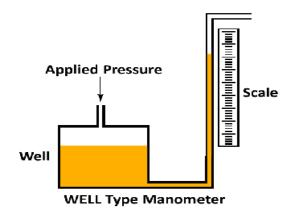
Thus, the well manometer provides an easier means of reading pressure. No longer does one have to measure the difference of height between two liquid columns, only the height of a single column.
