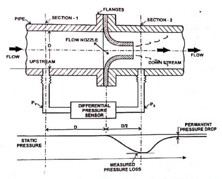
Figure 21.3: Flow nozzle arrangement
