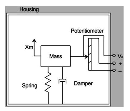
The natural frequency of these devices is generally less than 30 Hz, limiting their application to low frequency vibration measurements. Dynamic range is also limited. But they can measure down to 0 Hz (DC response).
