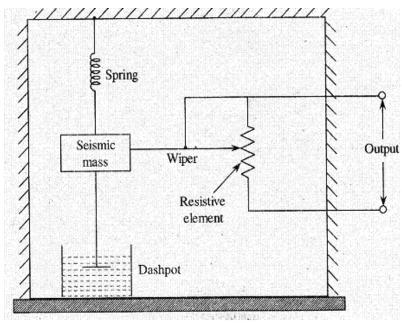
fig 9.1 Potentiometric accelerometer
