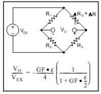
Figure 4. Quarter-Bridge Circuit
