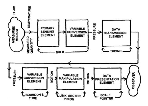
First Stage: The Detector-Transducer Stage
