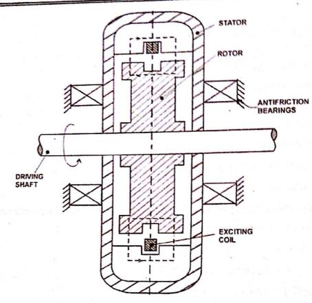
Figure 12.3: Eddy current dynamometer
