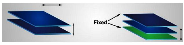
In these accelerometers, a diaphragm acting as a mass moves in the presence of acceleration. The diaphragm is sandwiched between the two fixed plates creating two capacitors; each with an individual fixed plate and each sharing the diaphragm as a movable plate. Movement of the diaphragm causes a capacitance shift by altering the distance between two parallel plates, the diaphragm itself being one of the plates.
