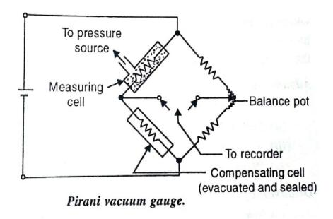
As the surrounding pressure changes, the filament temperature and hence its resistance also changes. A compensating cell is also employed to minimized variation caused by ambient temperature changes. The resistance change of the filament in the measuring cell is measured by the use of a resistance bridge which is calibrated in terms of pressure.
