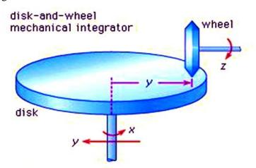
✓ Thus the rotations of the disk and the wheel are related through multiplicative factors and the number of turns made by the integrating wheel (for any number of turns of the disk) will be expressed as a definite integral of the function represented by the variable position of the wheel on the disk.
