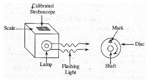
fig 10.1 Shaft Speed Measurement Using Stroboscope
