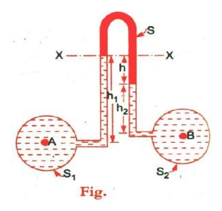
Let the pressure at the point A and B and PA and PB respectively
