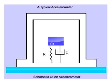
When the system is subjected to linear acceleration, a force (= mass \* acceleration) acts on the proof-mass. This causes it to deflect; the deflection is sensed by a suitable means and is converted into an equivalent electrical signal.
