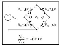
Figure 7. Full-Bridge Circuit
