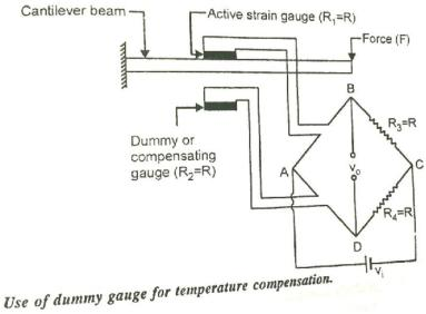
The bridge is initially balanced and therefore  $\frac{R_1}{R_2} = \frac{R_3}{R_4}$ . Suppose a change in temperature occurs,
