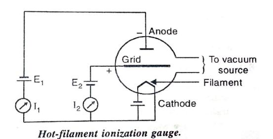
The grid draws electrons from heated filament and collision between them and gas molecules causes ionization of the molecules.as the plate is negatively charged, the positively charged ions are attached to the plate of the tube, causing current  $(I_1)$  flow in the external circuit. The electrons are collected by the grid and a current  $I_2$  is produced in the grid circuit.
