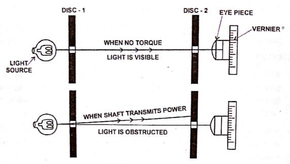
Figure 12.5: Flash light torsion dynamometer
