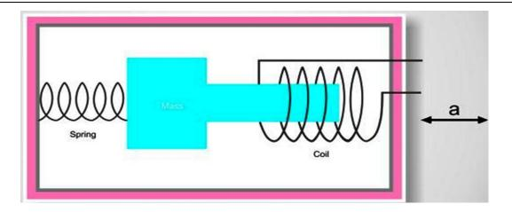
When the body is accelerated, the proof mass moves. In other words, portion of the core inside the coil changes and so the coil impedance. Thus, the coil impedance is a function of the applied acceleration.
