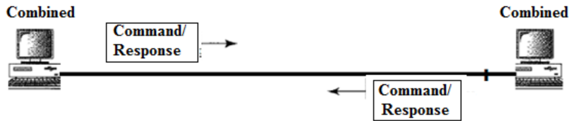
Figure 2.21 Asynchronous balanced mode
