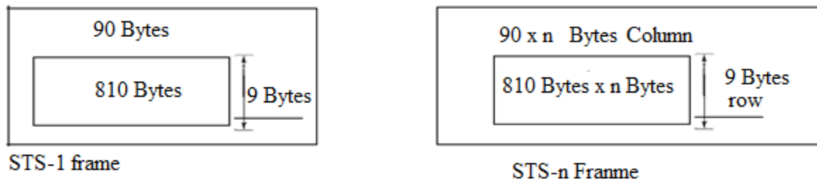
Figure 1.23 An STS-1 and STS-n Frame
