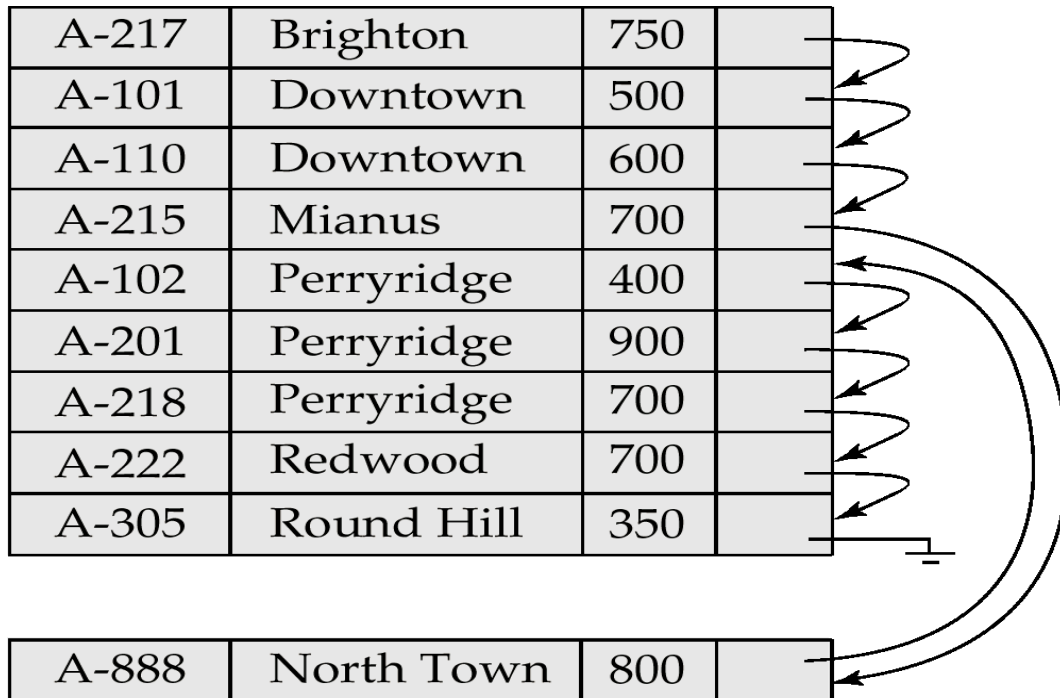
Fig. The role of Overflow block in sequential file organization
