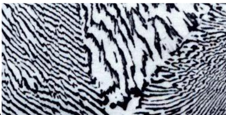
Figure 3. (A) Microstructure of a Pb-Sn eutectic with 61.9% Sn. (B) Microstructure of a Pb-Sn alloy of composition 60 wt.% Sn; with proeutectic \alpha phase and eutectic. The dark regions are Pb-rich \alpha phase; the bright areas are Sn-rich \beta phase. (From Callister).
