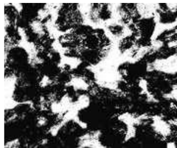
Figure 9 Photomicrograph of White Cast Iron
