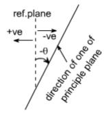
Therefore the direction of other principal planes would be  $\{<< +90\}$  since the angle << is always less in magnitude then 90 hence the quantity (<<< +90) would be positive therefore the Inclination of other plane with reference plane would be positive therefore if just complete the Block. It would appear as
