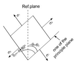
If we just want to measure the angles from the reference plane, than rotate this block through 180<sup>0</sup> so as to have the following appearance.
