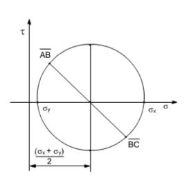
(4) As already defined the principal planes are the planes on which the shear components are zero.
