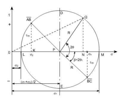
Consider any point Q on the circumference of the circle, such that PQ makes an angle 2<< with BC, and drop a perpendicular from Q to meet the s axis at N.Then OQ represents the resultant stress on the plane an angle < to BC. Here we have assumed that  $<_x < < <_y$
