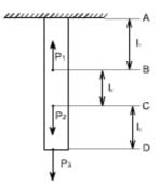
When either the axial force or the cross – sectional area varies continuosly along the axis of the bar, then equation (1) is no longer suitable. Instead, the elongation can be found by considering a deferential element of a bar and then the equation (1) becomes
