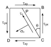
Complementary shear stresses of equal value but of opposite effect are then set up on the sides AD and BC in order to prevent the rotation of the element. Since the applied and complementary shear stresses are of equal value on the x and y planes. Therefore, they are both represented by the symbol  $\tau_{xy}$ .
