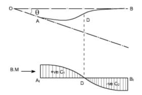
Then, adequate precaution must be exercised in using the above theorem. In such a case B. M diagram gets divide into two portions +ve and –ve portions with centroids  $C_1$  and  $C_2$ . Then to find an angle < between the tangents the points A and B
