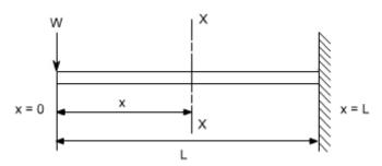
In order to solve this problem, consider any X-section X-X located at a distance x from the left end or the reference, and write down the expressions for the shear force abd the bending moment
