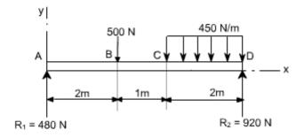
As an clear indication of these restrictions, one may use a nomenclature in which the usual form of parentheses is replaced by pointed brackets, namely,  $\leftrightarrow$ . With this change in nomenclature, we obtain a single moment equation
