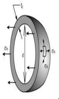
Because of the symmetry of the sphere the stresses set up owing to internal pressure will be two mutually perpendicular hoops or circumferential stresses of equal values. Again the radial stresses are neglected in comparison to the hoop stresses as with this cylinder having thickness to diametre less than1:20.
