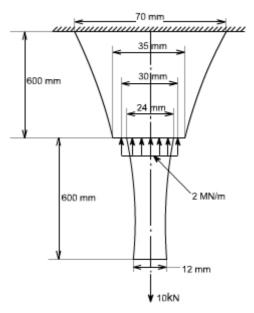
**Example 2:** A round bar, of length L, tapers uniformly from radius  $r_1$  at one end to radius  $r_2$  at the other. Show that the extension produced by a tensile axial load P
