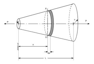
consider the above figure let  $r_1$  be the radius at the smaller end. Then at a X crosssection XX located at a distance x from the smaller end, the value of radius is equal to
