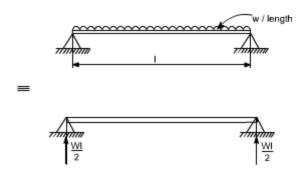
In order to write down the expression for bending moment consider any crosssection at distance of x metre from left end support.
