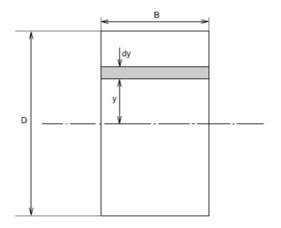
Consider the rectangular beam cross-section as shown above and an element of area dA, thickness dy, breadth **B** located at a distance **y** from the neutral axis, which by symmetry passes through the centre of section. The second moment of area **I** as defined earlier would be
