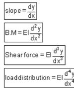
**Methods for finding the deflection:** The deflection of the loaded beam can be obtained various methods. The one of the method for finding the deflection of the beam is the direct integration method, i.e. the method using the differential equation which we have derived.
