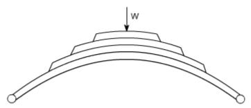
These type of springs are used in the automobile suspension system.
