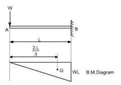
Let us workout this problem from the zero slope condition and apply the first area - moment theorem
