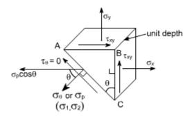
Consider once again the equilibrium of a triangular block of material of unit depth, Assuming AC to be a principal plane on which principal stresses  $<_p$  acts, and the shear stress is zero.
