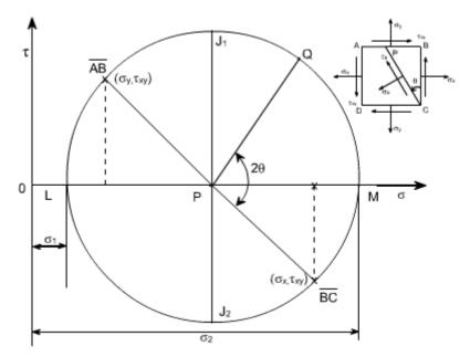
As we know that the circle represents all possible states of normal and shear stress on any plane through a stresses point in a material. Further we have seen that the co-ordinates of the point 'Q' are seen to be the same as those derived from equilibrium of the element. i.e. the normal and shear stress components on any plane passing through the point can be found using Mohr's circle. Worthy of note:
