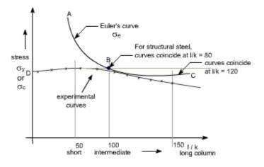
Allowing for the imperfections of loading and strut, actual values at failure must lie within and below line CBD.
