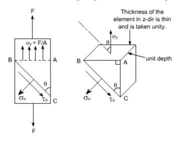
The stress acting at a point is represented by the stresses acting on the faces of the element enclosing the point. The stresses change with the inclination of the planes passing through that point i.e. the stress on the faces of the element vary as the angular position of the element changes. Let the block be of unit depth now considering the equilibrium of forces on the triangle portion ABC. Resolving forces perpendicular to BC, gives
