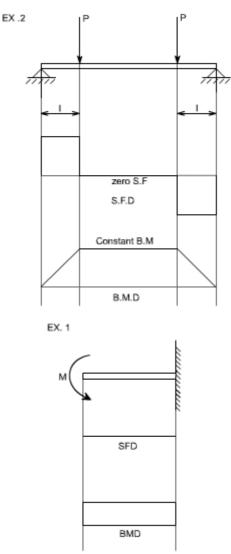
When a beam is subjected to pure bending are loaded by the couples at the ends, certain cross-section gets deformed and we shall have to make out the conclusion that,
