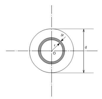
Consider any circular strip of thickness < r located at a radius 'r'.
