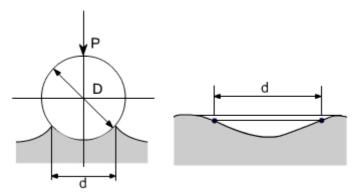
After removing the load an indentation remains on the surface of the test specimen. If area of the spherical surface in the indentation is denoted as F sq. mm. Brinell Hardness number is defined as :
