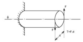
Effects of Torsion: The effects of a torsional load applied to a bar are
