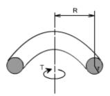
In this case the material of the spring is subjected to pure bending which tends to reduce Radius R of the coils. In this case the bending moment is constant throughout the spring and is equal to the applied axial Torque T. The stresses i.e. maximum
