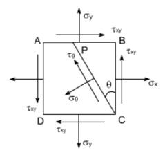
As per the double subscript notation the shear stress on the face BC should be notified as  $<_{yx}$ , however, we have already seen that for a pair of shear stresses there is a set of complementary shear stresses generated such that  $<_{yx} = <_{xy}$
