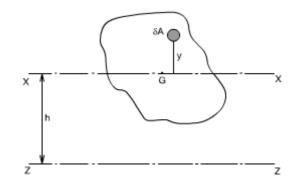
If 'ZZ' is any axis in the plane of cross-section and 'XX' is a parallel axis through the centroid G, of the cross-section, then
