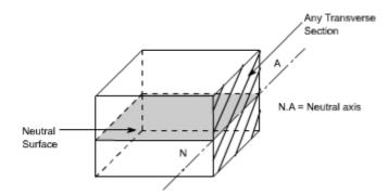
We know that when a beam is under bending the fibres at the top will be lengthened while at the bottom will be shortened provided the bending moment M acts at the ends. In between these there are some fibres which remain unchanged in length that is they are not strained, that is they do not carry any stress. The plane containing such fibres is called neutral surface.
