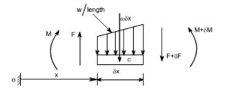
The forces acting on the free body diagram of the detached portion of this loaded beam are the following
