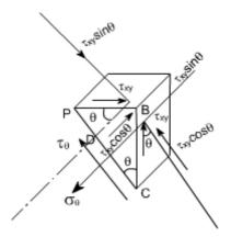
Assuming unit depth and resolving normal to PC or in the direction of  $\sigma_{ heta}$
