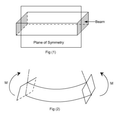
When a member is loaded in such a fashion it is said to be in **<u>pure bending</u>**. The examples of pure bending have been indicated in EX 1 and EX 2 as shown below :
