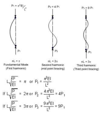
If load is applied sufficiently quickly to the strut, then it is possible to pass through the fundamental mode and to achieve at least one of the other modes which are theoretically possible. In practical loading situations, however, this is rarely achieved since the high stress associated with the first critical condition generally ensures immediate collapse.
