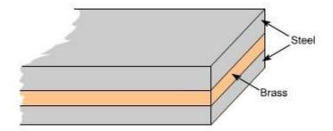
If we have both applied stresses and a temp. change, thermal strains may be added to those given by generalized hook's law equation –e.g.
