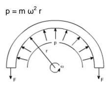
Fig 19.1: Thin ring rotating with constant angular velocity
