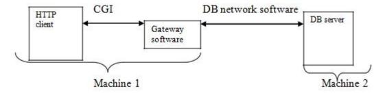
**High-level details of using CGI and gateway software-** Processing software is called directly from the HTML search document by the HTTP client. The processing software reads the query input passes to it via the CGI call.
