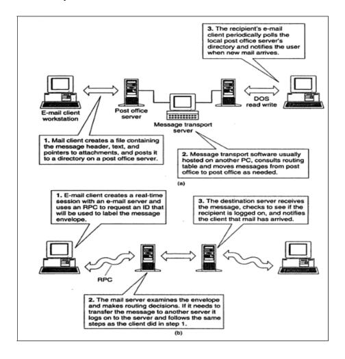
**Figure:** How E-Mail works three staps to mail delivery: (a) File-Based systems; (b) Client/Server-Based systems.
