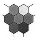
Figure 2.1 A hexagonal array of seven cells using seven different channels
