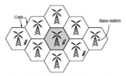
Figure. Cellular design of mobile phone networks
