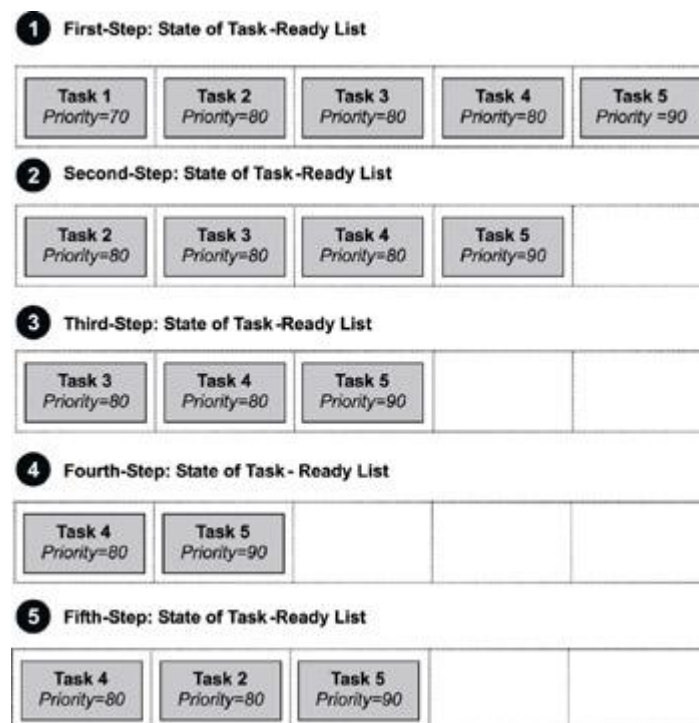
Figure 3: Five steps showing the way a task-ready list works.
