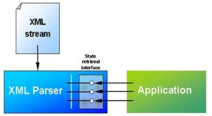
Fig 1.20 Working of XML Parser with inteface
