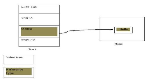
Fig 1.5 Stack and Heap
