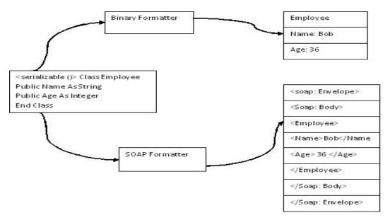
The figure illustrates the serialization process. As the figure shows, an instance of a class can be run through a formatter that extracts the state of this object in a particular form. The binary formatter emits that state information in a simple and
