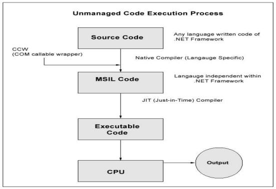
Fig1.10 Unmanaged Code Execution Process
