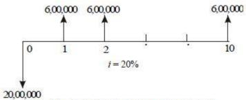
Fig. 4.4 Cash flow diagram for technology 2.
