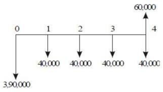
Fig. 6.13 Cash flow diagram for alternative 1.
