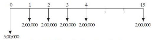
Fig. 6.4 Cash flow diagram for manufacturer 1.
