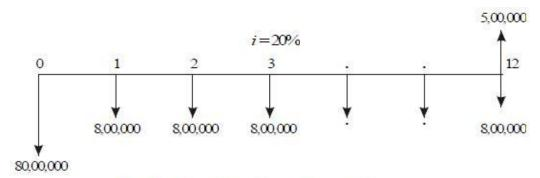
Fig. 5.9 Cash flow diagram for manufacturer 1.
