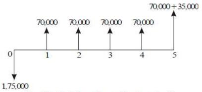
Fig. 6.8 Cash flow diagram for alternative B.
