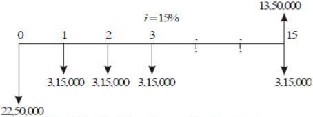
Fig. 6.11 Cash flow diagram for alternative 1
