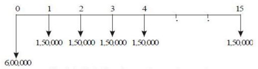
Fig. 6.6 Cash flow diagram for manufacturer 3.
