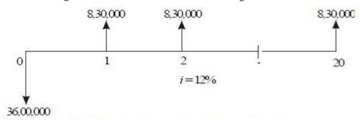
Fig. 5.6 Cash flow diagram for alternative 2.
