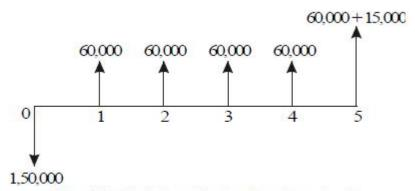
Fig. 6.7 Cash flow diagram for alternative A.
