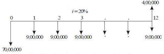
Fig. 5.10 Cash flow diagram for manufacturer 2.
