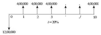
Fig. 4.3 Cash flow diagram for technology 1.
