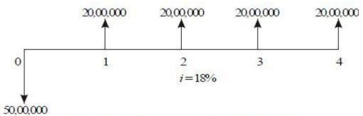
Fig. 5.3 Cash flow diagram for alternative A.
