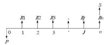
Fig. 7.1 Generalized cash flow diagram.
