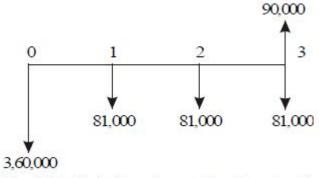
Fig. 6.14 Cash flow diagram for alternative 2.
