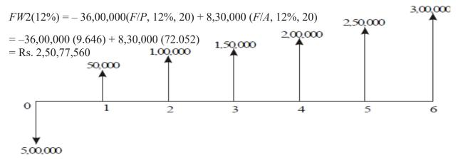
Fig. 5.7 Cash flow diagram for alternative 1.
