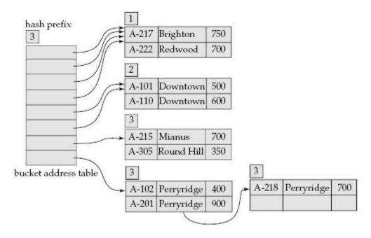
Figure 12.31 Extendable hash structure for the account file.
