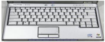
On portable systems, such as laptops and notebooks, the keyboard can be a crucial part of the product evaluation process for two reasons: the keyboard is integrated into the unit and is not easily replaceable and the smaller size of the keyboard often forces to fit all the keys into the space provided in it. The function keys are here integrated with the alphabetic key itself. Using NUM LOCK, we can use those keys.
