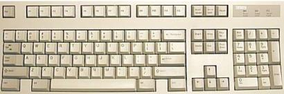
The Enhanced 101-key keyboard is the most familiar to computer used today. Here only 101 keys are used and placed in the keyboard. Function keys are increased into 12 (i.e.) F1 to F12. Those keys are placed in the horizontal row above the number keys, with a ESC key in its upper left corner position. A second CTRL and second ALT key is added to the bottom of row. Here cursor keys are available in an inverted  $-T\parallel$  formation and the other navigation keys.
