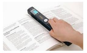
Portable scanners are small enough to bring on the road. In fact, some are small enough to put in your pocket; pen scanners are just a bit bigger than fountain pens and can scan the text of a document line by line. Some are as wide as a page and roll easily down the page. They're not going to give high-resolution scans and so aren't good for scanning photographs or other applications where you need a high-quality result. Since they're not cheaper than flatbed scanners.
