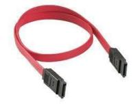
SATA host-adapters and devices communicate via a high-speed serial cable over two pairs of conductors. In contrast, parallel ATA (the redesignation for the legacy ATA specifications) used a 16bit wide data bus with many additional support and control signals, all operating at much lower frequency. To ensure backward compatibility with legacy ATA software and applications, SATA uses the same basic ATA and ATAPI command-set as legacy ATA devices.
