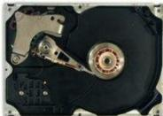
*The inside of a hard disk drive with the disk itself removed. To the left is the read-write arm. In the middle the electromagnets of the platter's motor can be seen.*
