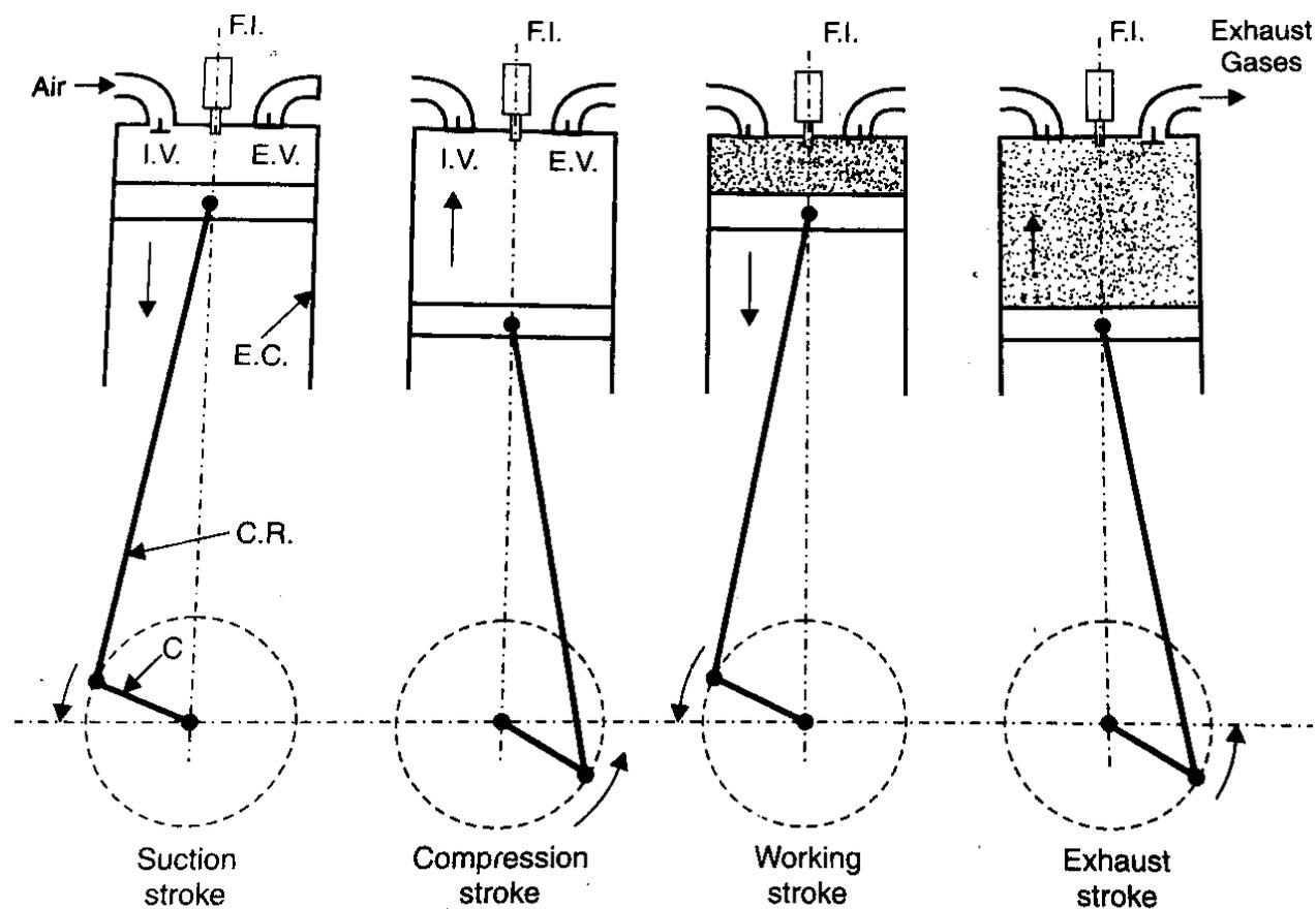
F.I. = Fuel injector ; I.V. = Inlet valve ; E.V. = Exhaust valve.
