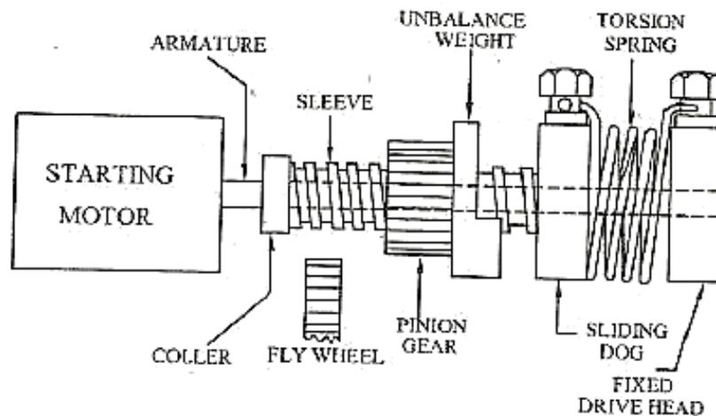
When the motor starts, the armature shaft rotates. Due to the unbalance weight, the pinion cannot rotate and it moves axially towards the motor. The pinion is engaged with flywheel. There is collar attached on the sleeve. Now the pinion is engaged and rotates the flywheel of the engine and the engine starts. When the engine starts, the self-starter switch is off.
