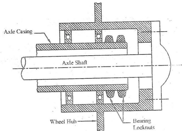
The axle shaft is not supported by bearings but it is positioned at its ends. Hence, in this method, the axle is relieved of all strains due to the load of the vehicle or end thrust. Being free from all other strains, its duty is only to transmit a rotary motion to the wheel. Without disturbing the axle hub and the wheel, the axle shaft can be removed from the casing.
