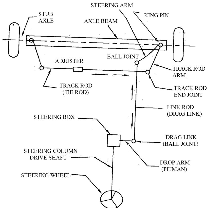
When the steering wheel is rotated the drop arm moves towards or away from the front wheel depending upon the direction of turn right or left
