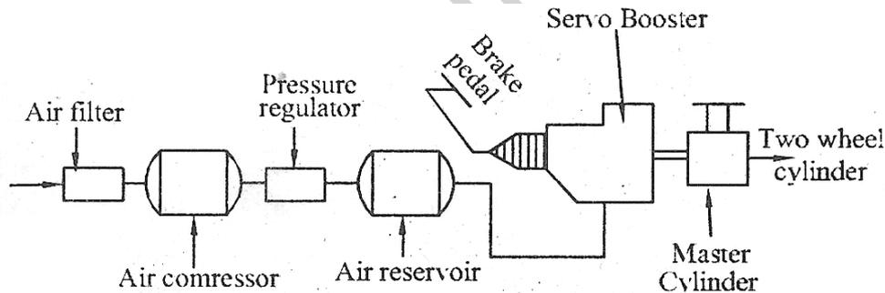
In vacuum assisted brake, vacuum was taken for pushing the push rod of the master cylinder. In air assisted hydraulic brake system instead of vacuum, air is used for application of brakes. The brake pedal link and push rod of master cylinder are so designed and linked that in the event of failure of air pressure, brakes can be applied but once again more foot pressure will be required.
