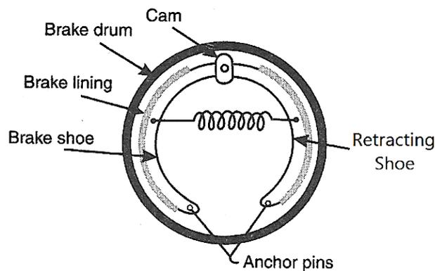
Mechanical Brakes (Cam - Operated)
