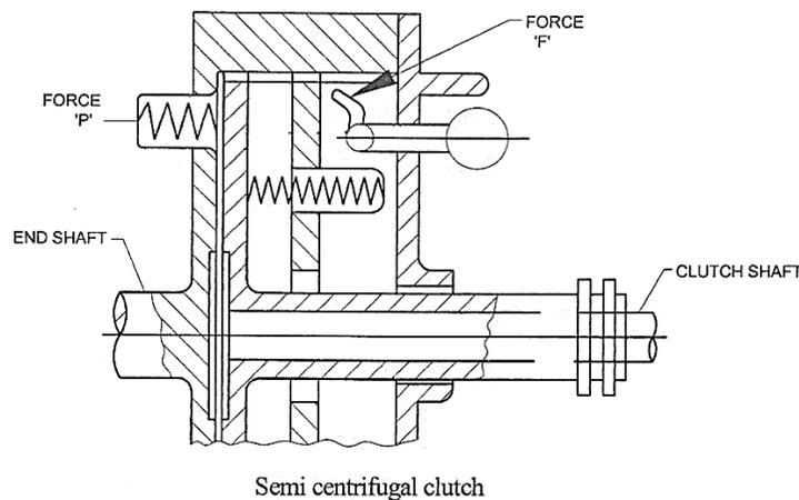
However at higher speeds, the weight C, due to the centrifugal force moves about A as fulcrum thereby pressing the pressure plate. The centrifugal force is proportional to the square of the speed so that adequate pressure level is attained. Fig. Shows the variation of force on the pressure plate at various speeds
