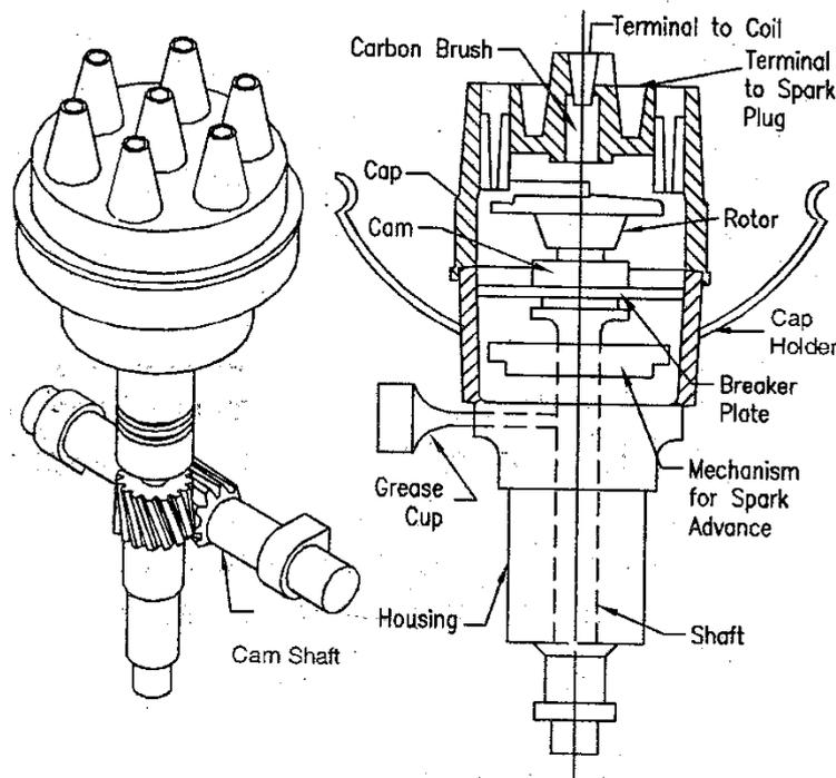
The H.T cables lead the high voltage to the spark plug. The central terminal is connected to the secondary of the ignition coil. As the distributor spindle has to rotate at half the crank shaft speed, the drive for it is taken from the cam shaft through spiral gears. As the distributor spindle rotates, the rotor point comes into contact with each terminal in the cap. Thus the high voltage passes to each cylinder in turn. Fig. shows the exploded view of distributor.
