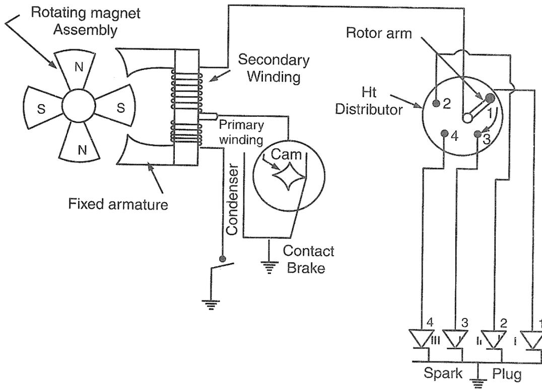
Magneto ignition system for a four cylinder engine
