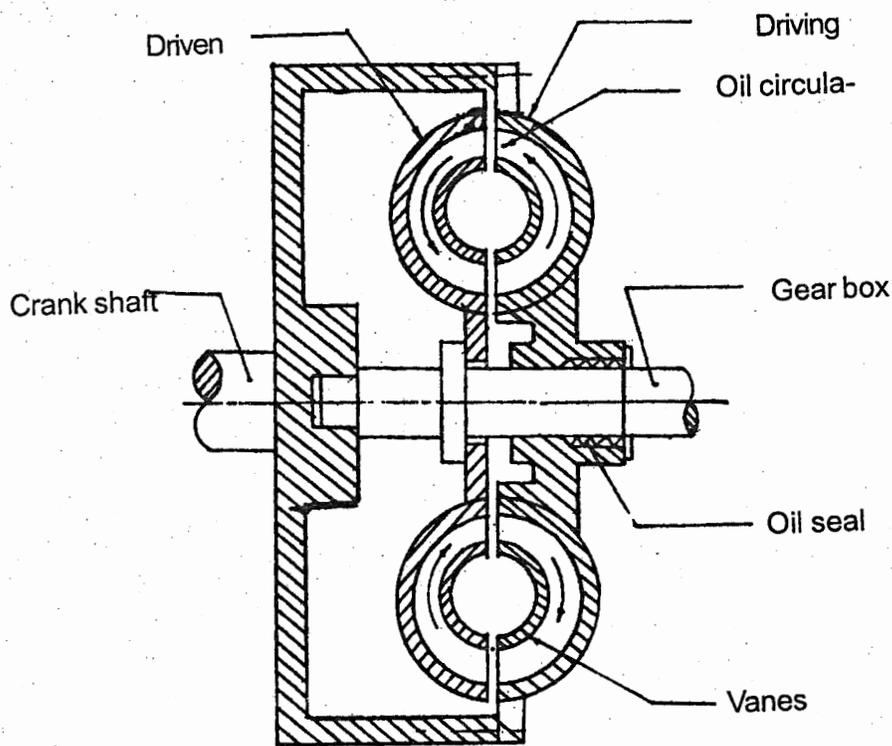
The oil is thrown out against the curved interior surface because of a centrifugal force. Then, it is directed across, to the runner and returned to the impeller. When the efficiency of the coupling is highest, under best operating conditions, runner speed is almost equal to the impeller. The lagging of the driven unit behind the driver unit is known as slip.
