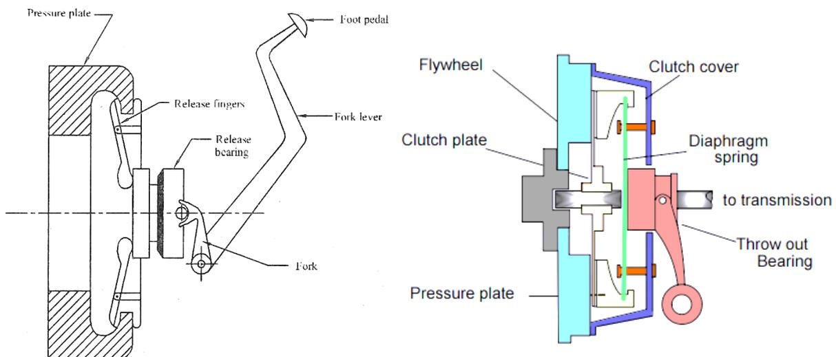
It consists of the foot pedal, Fork lever, Fork, thrust bearing and fingers as shown in fig. The release bearing is held in a fork and is free to move over the clutch shaft. The fork in turn is connected with the foot pedal through the fork lever. The thrust bearing operates the clutch release fingers provided in the pressure plate.
