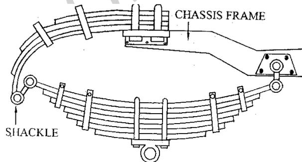
It is a combination of semi-elliptical and quarter elliptical spring. In the olden days it was popular but has been now replaced by semi-elliptical spring
