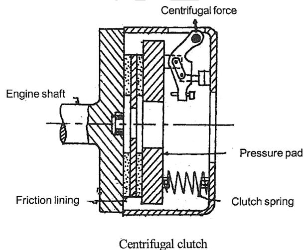
As the speed increases, the fly-weights move outwards due to centrifugal force. This movement operates a bell crank lever and presses the floating plate. As shown in the figure, there are helical springs between the floating plate and pressure plate. The force is transmitted to the pressure plate through the springs.
