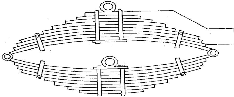
Full elliptical spring consist of two semi-elliptical springs joined together oppositely. This type of spring was used in old cars. They do not maintain correct axle alignment.
