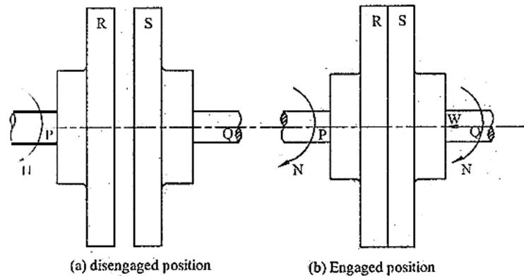
Principle of Friction Clutches.
