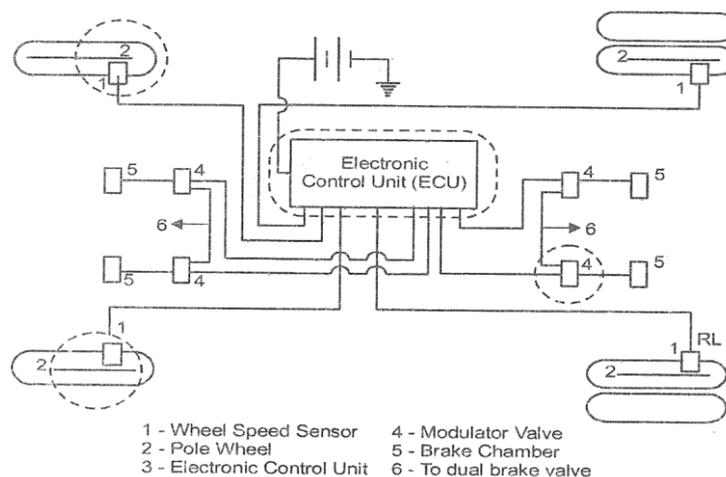
Anti-lock braking system
