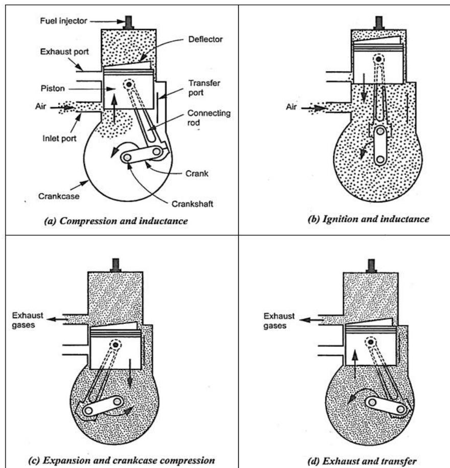
**Two Stroke - Diesel Engine**
