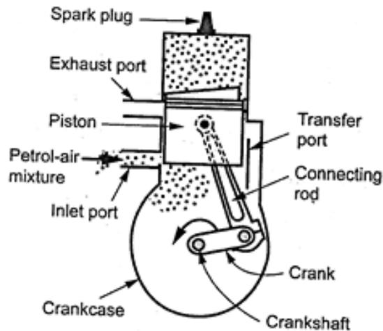
The crown of the piston (i.e., top of the piston) is shaped in such a way to assist in deflecting the fresh charge upwards in the cylinder and help scavenging.
