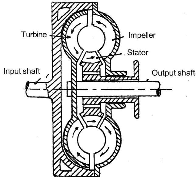
Fig. Torque converter
