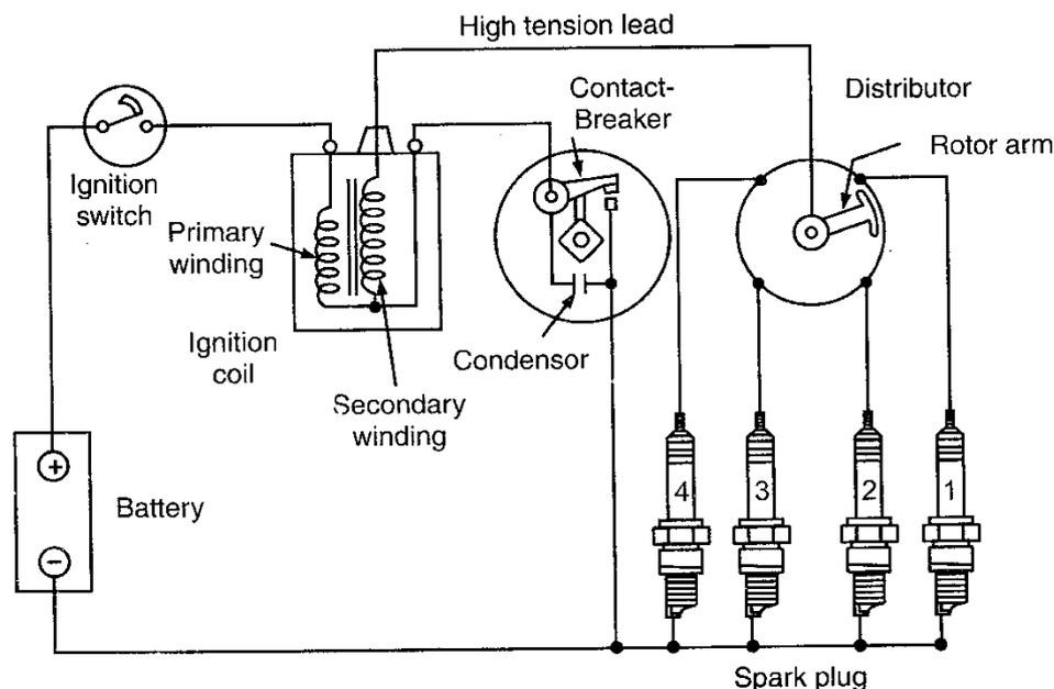
Battery ignition system for four-cylinder engine
