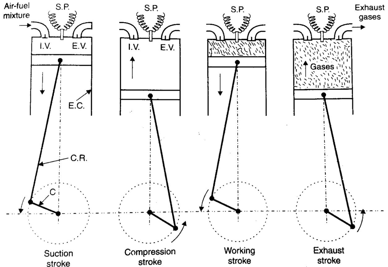
I.V. = Inlet valve ; E.V. = Exhaust valve ; E.C. = Engine cylinder ; C.R. = Connecting rod ;
