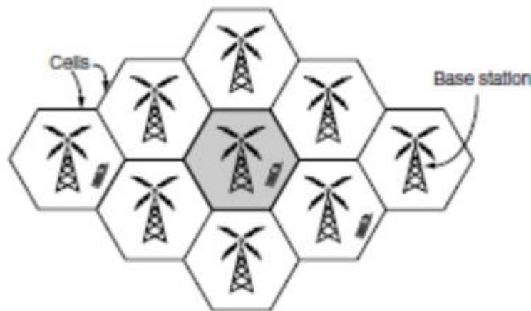
**Figure.** Cellular design of mobile phone networks
