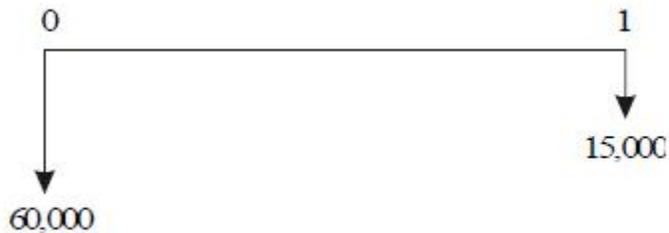
**Fig. 6.19** Cash flow diagram for alternative 1.
