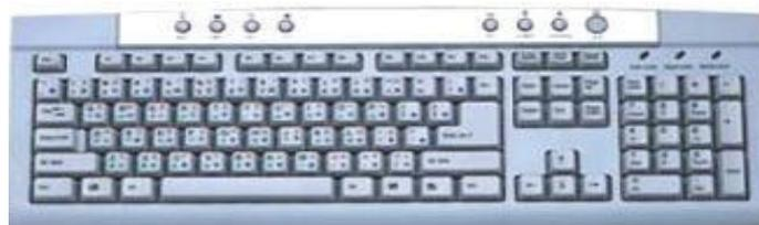
This is identical to the 101 – key layouts, except for the addition of three keys: Two windows keys which is located between the CTRL and ALT keys on both sides and an Application key on the right side, next to the window key. By pressing the window key at any time we can open the start menu, and pressing the application key displays the context menu for currently highlighted item.
