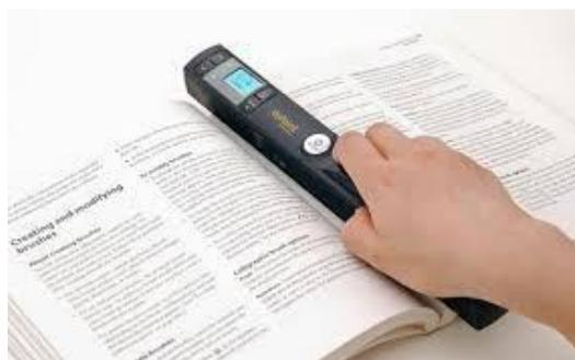
Portable scanners are small enough to bring on the road. In fact, some are small enough to put in your pocket; pen scanners are just a bit bigger than fountain pens and can scan the text of a document line by line. Some are as wide as a page and roll easily down the page. They're not going to give high-resolution scans and so aren't good for scanning photographs or other applications where you need a high-quality result. Since they're not cheaper than flatbed scanners.
