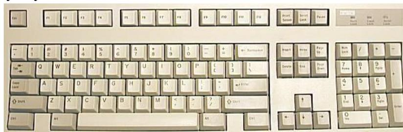
The Enhanced 101-key keyboard is the most familiar to computer used today. Here only 101 keys are used and placed in the keyboard. Function keys are increased into 12 (i.e.) F1 to F12. Those keys are placed in the horizontal row above the number keys, with a ESC key in its upper left corner position. A second CTRL and second ALT key is added to the bottom of row. Here cursor keys are available in an inverted -T formation and the other navigation keys.
