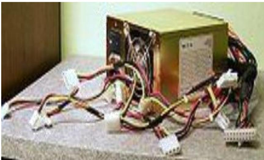
**12V only** power connector (labelled **P1**, though it is not compatible with the ATX 20 or 24 pin connector): This is a 16-pin Molex connector supplying the motherboard with six 12V lines with common returns, a 'supply OK' signal, a 'PSU ON' signal and an 11V auxiliary supply. One pin is left unused.<sup>[15]</sup>
