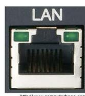
If there are no lights or the lights are orange or red, the card may be bad, not connected properly, or may not be receiving a signal from the network. If you are on a small or local network and have the capability of checking a hub, switch, or router, verify that the cables are properly connected and that it has power. If after checking the connections, the LED indicators appear bad, the network adapter, port, or cable may be defective.
