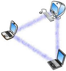
An ad-hoc or peer-to-peer wireless network consists of a number of computers each equipped with a wireless networking interface card. Each computer can communicate directly with all of the other wireless enabled computers. They can share files and printers this way, but may not be able to access wired LAN resources, unless one of the computers acts as a bridge to the wired LAN using special software.
