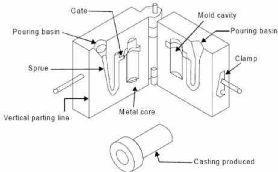
*Fig. 4.1 A typical permanent mould*
