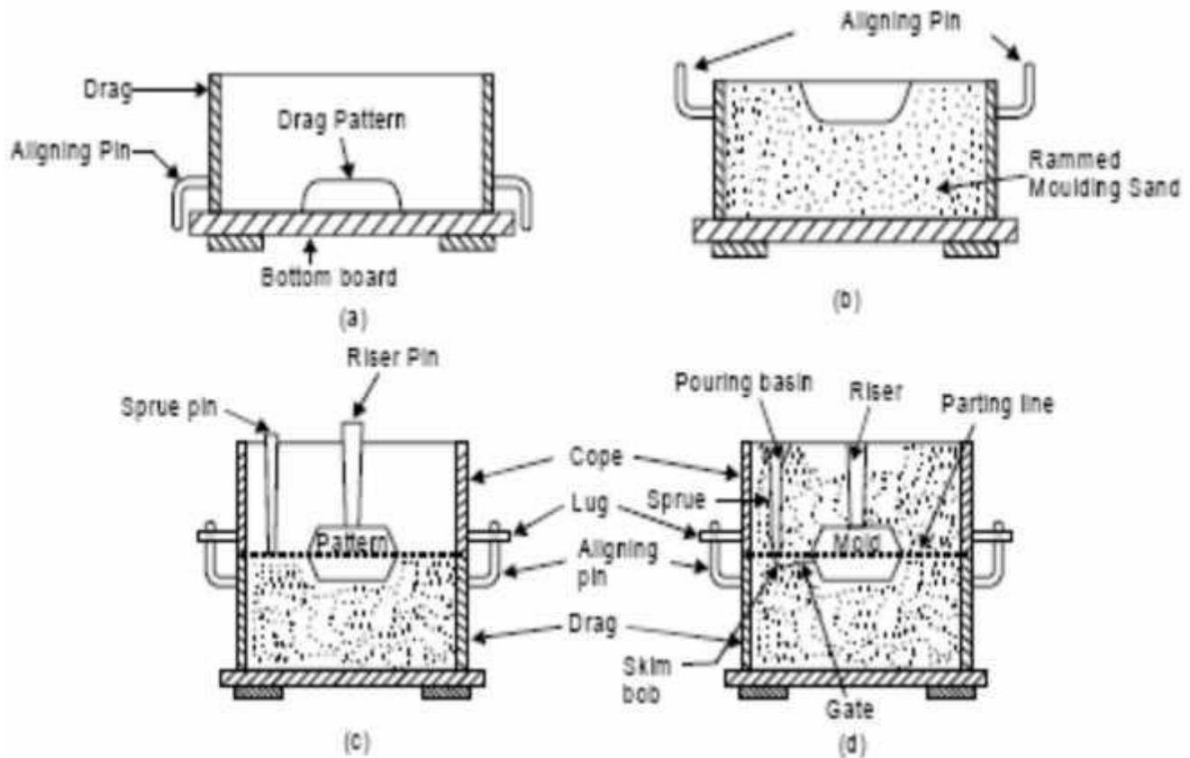
*Fig. 1.27 Mould making*
