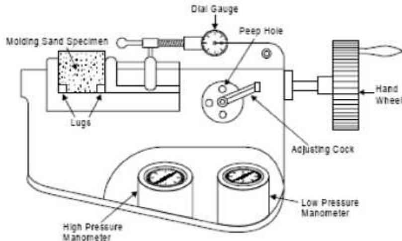
*Fig. 1.23 Strength testing machine*
