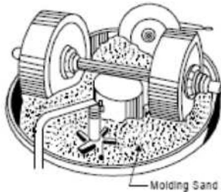
*Fig. 1.26 Sand mixing muller*
