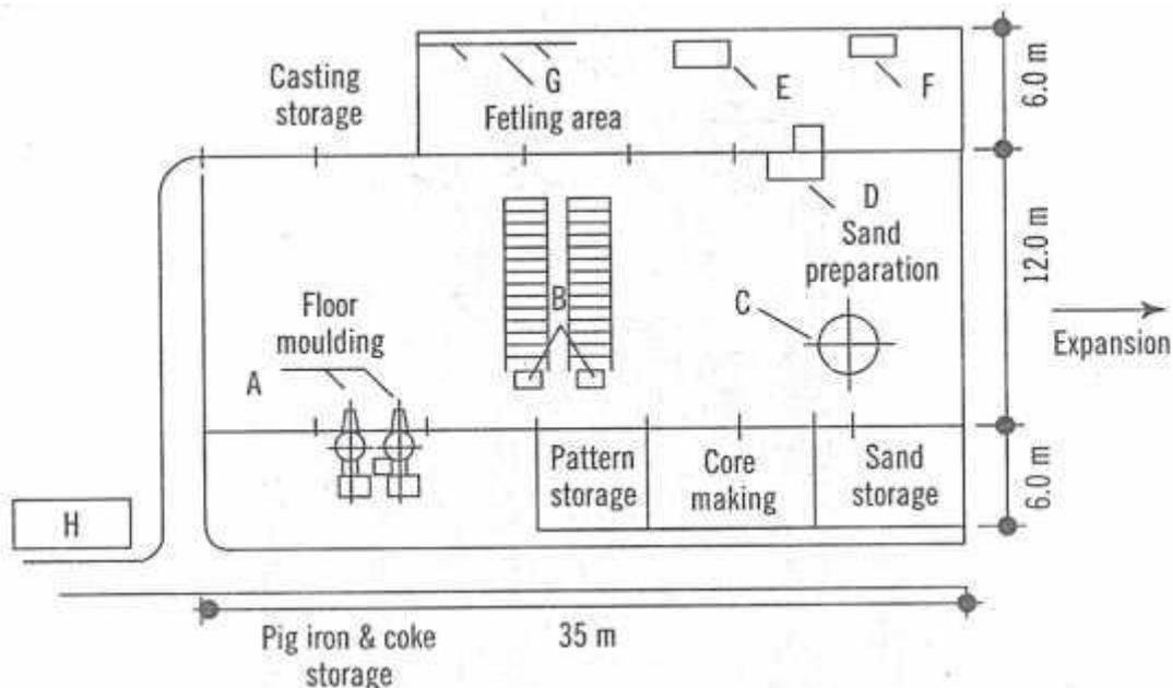
*Fig. 5.11 Layout of a small grey iron foundry*
