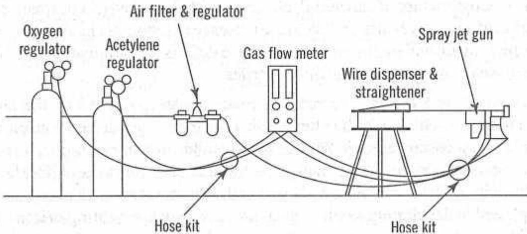
*Fig. 5.4 Set-up for metal spraying*
