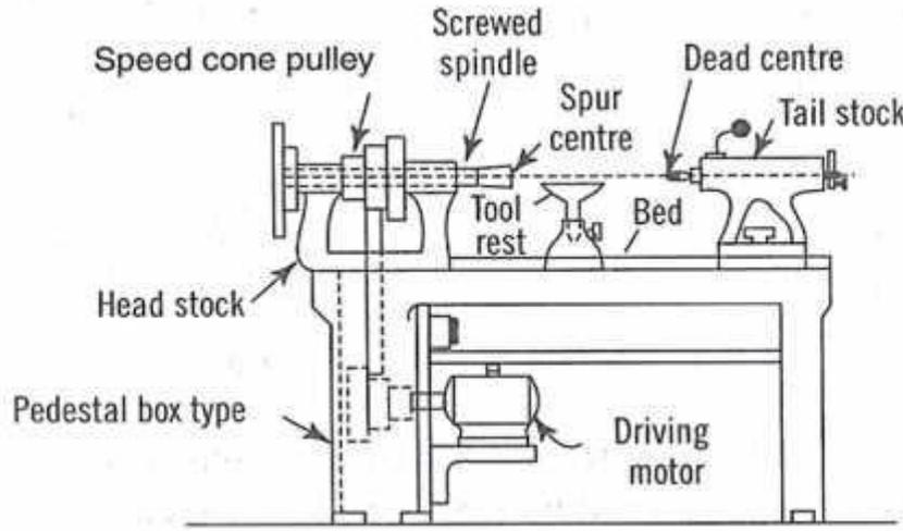
*Fig 1.3 Woodworking lathe*
