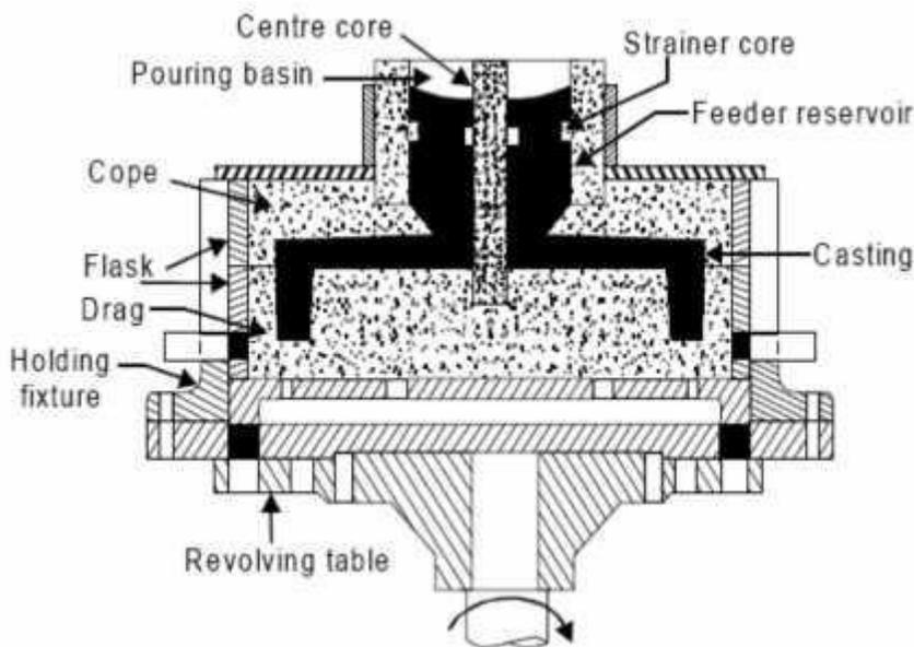
Fig. 4.9 Semi-centrifugal casting setup
