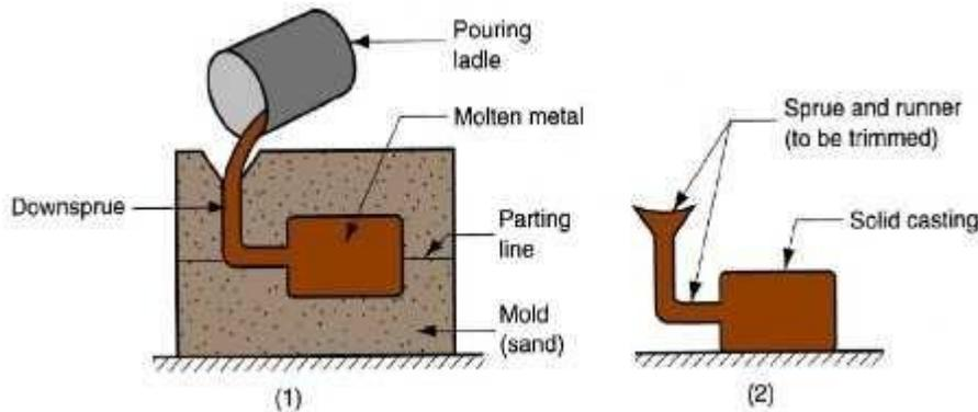
*Fig 1.1 Casting Process*
