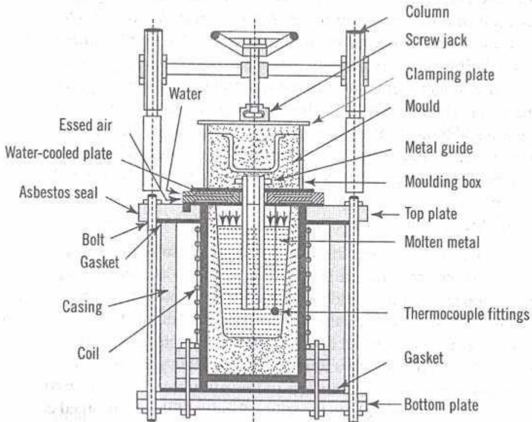
*Fig. 4.6 Low-pressure die-casting machine*
