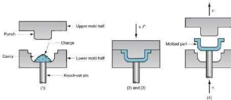
*Fig. 4.15 Compression moulding for thermosetting plastics: (1) charge is loaded; (2) and (3) charge is compressed and cured; and (4) part is ejected and removed (some details omitted)*
