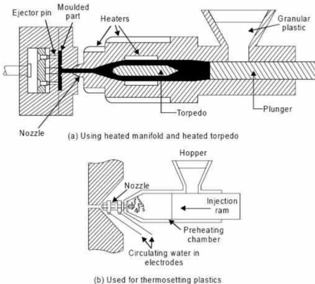
*Fig. 4.17 Typical injection moulding*
