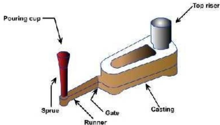
*Fig 1.2 a typical pattern attached with gating and risering system*
