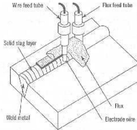
*Fig. 5.1 Submerged Arc Welding*
