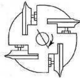
*Fig 1.7 Cross section of cutter*
