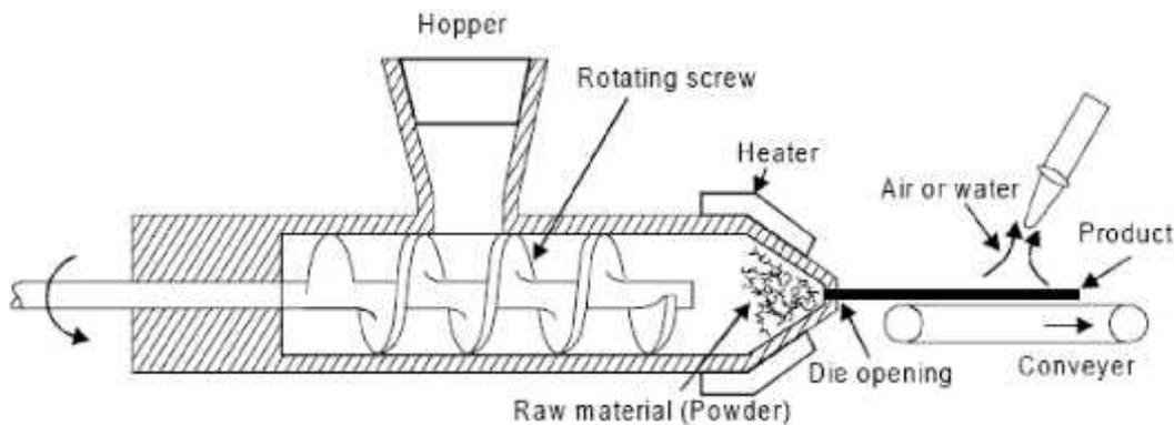
*Fig. 4.18 Schematic extrusion moulding*
