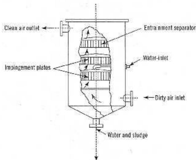
*Fig. 5.9 Wet centrifugal dust collector*
