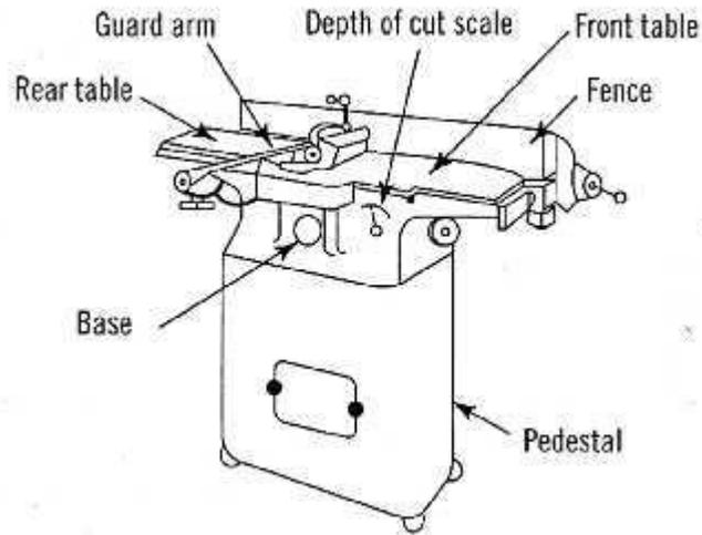
*Fig 1.5 Wood Jointer*
