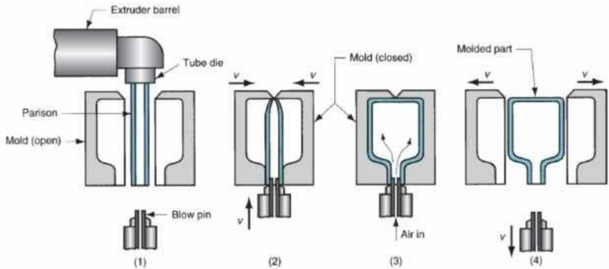
*Fig. 4.19 Extrusion blow moulding: (1) extrusion of parison; (2) parison is pinched at the top and sealed at the bottom around a metal blow pin as the two halves of the mould come together; (3) the tube is inflated so that it takes the shape of the mould cavity; and (4) mould is opened to remove the solidified part.*
