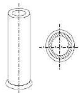
Fig. 4.8 Article produced by true centrifugal casting process
