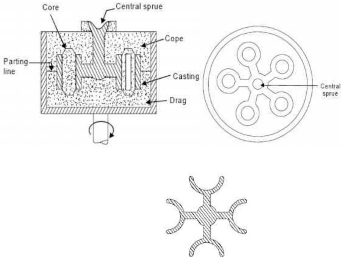
*Fig. 4.11 Centrifuging casting setup*
