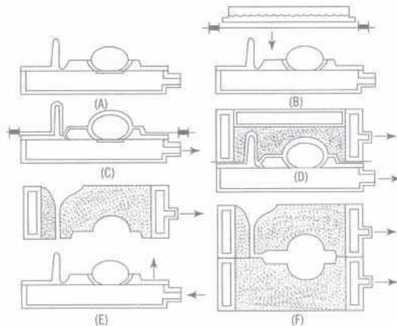
*Fig. 4.14 Steps in vacuum moulding process*
