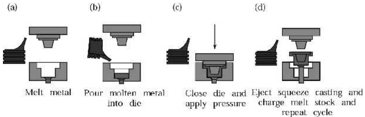
*Sequence of operations in the squeeze-casting process.*
