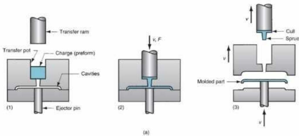
*Fig. 4.16 (a) Pot transfer moulding, and (b) plunger transfer moulding.*
