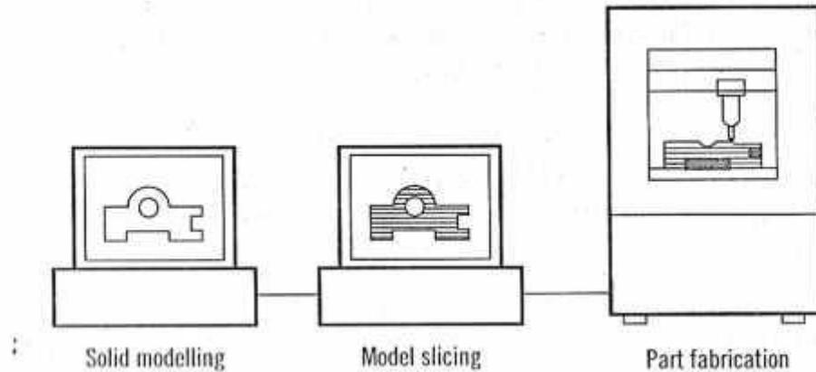
*Fig 1.11 Main steps in rapid prototyping*
