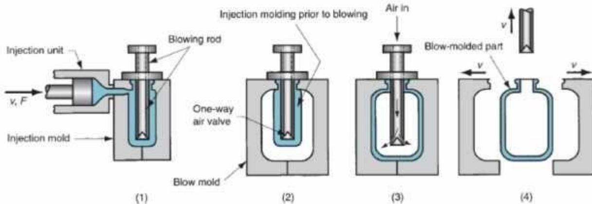
*Fig. 4.20 Injection blow moulding: (1) parison is injected moulded around a blowing rod; (2) injection mould is opened and parison is transferred to a blow mould; (3) soft polymer is inflated to conform to the blow mould; and (4) blow mould is opened, and blown product is removed.*
