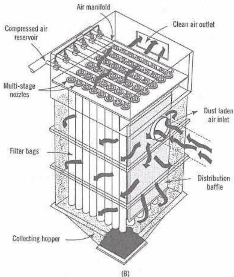
*Fig. 5.7 (A) Bag filter (B) Schematic arrangement of an ultra-jet type filter*
