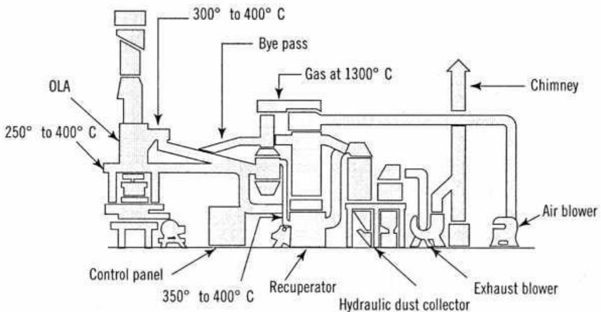
Fig. 5.10 Cupola furnace installation
