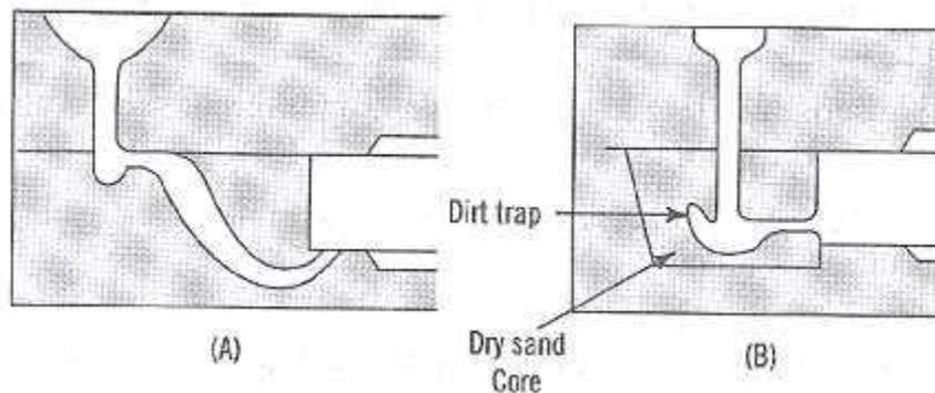
*Fig. 3.8 Types of bottom gates (A) Horn gate (B) Bottom gate with dry sand core*
