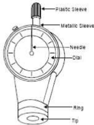
Fig. 1.25 Mould hardness tester
