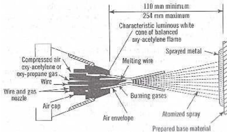
Fig. 5.3 Metal Spraying
