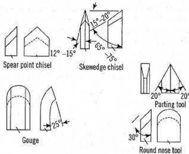
*Fig 1.4 woodworking lathe tools*
