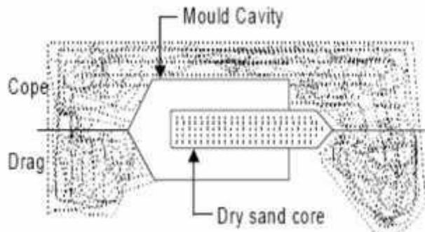
*Fig. 1.30 Balanced core*
