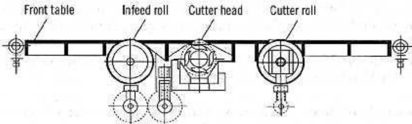
*Fig 1.6 Principle parts of a wood Planer*
