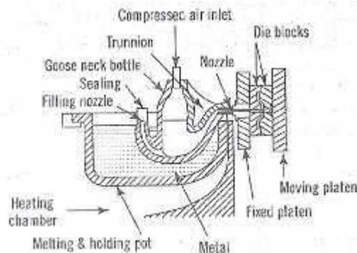
*Fig. 4.5 Air-blow type die-casting machine*
