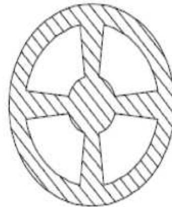
Fig. 4.10 Article produced by semicentrifugal casting process
