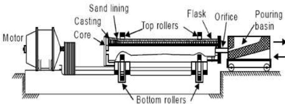
Fig. 4.7 De Levauud type true centrifugal casting process.
