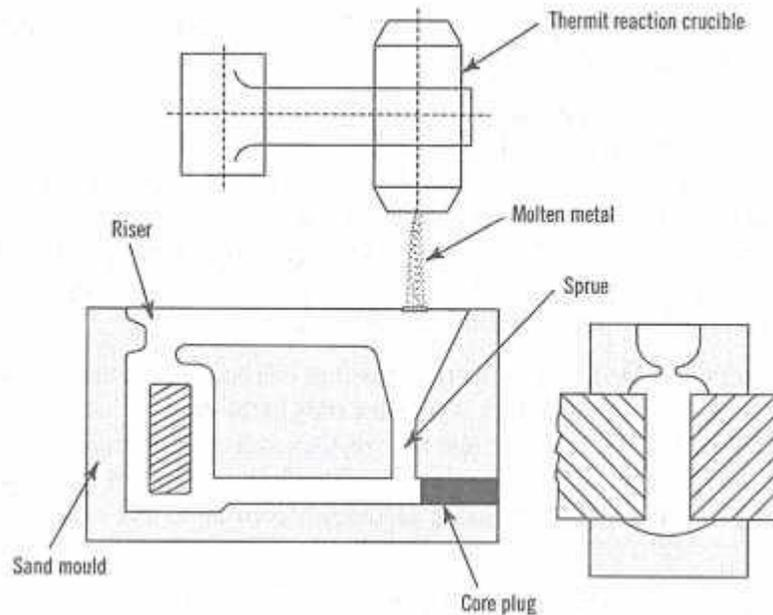
Fig. 5.2 Arrangement of thermit welding for casting repair
