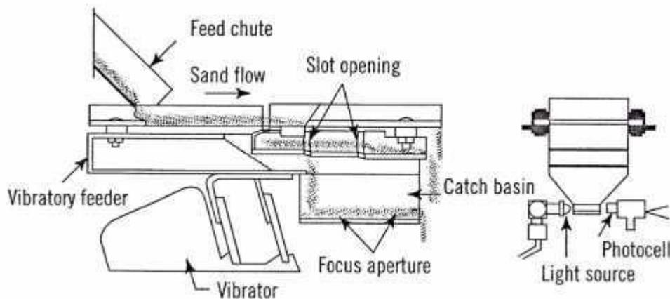
*Fig. 5.15 Mouldability Controller*
