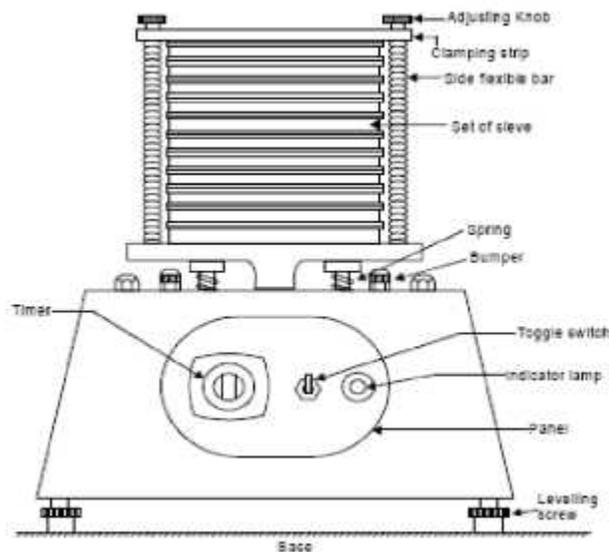
*Fig. 1.22 Grain fineness testing mechanical shaker*
