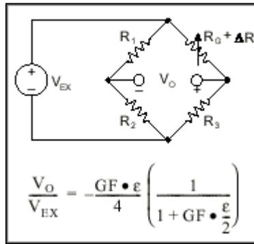
**Figure 4. Quarter-Bridge Circuit**
