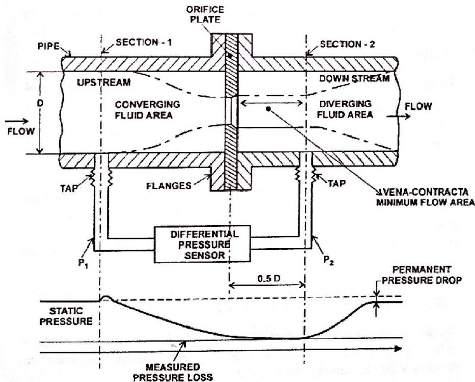
Figure 21.2: Orifice flow meter
