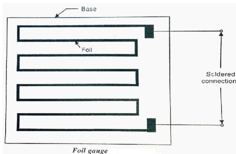
In these gauges, the bonding is better due to large surface area of the foil. The bonded foil gauges find a wider field of action.
