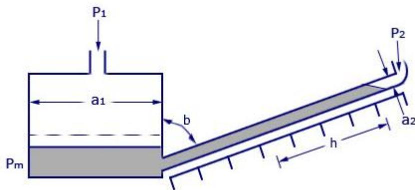
Inclined Tube manometer
