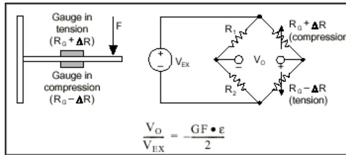
**Figure 6. Half-Bridge Circuit**
