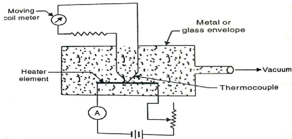
*Thermocouple vacuum gauge.*
