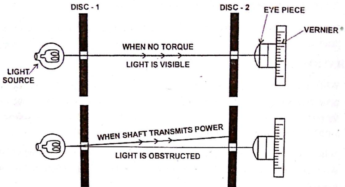
Figure 12.5: Flash light torsion dynamometer
