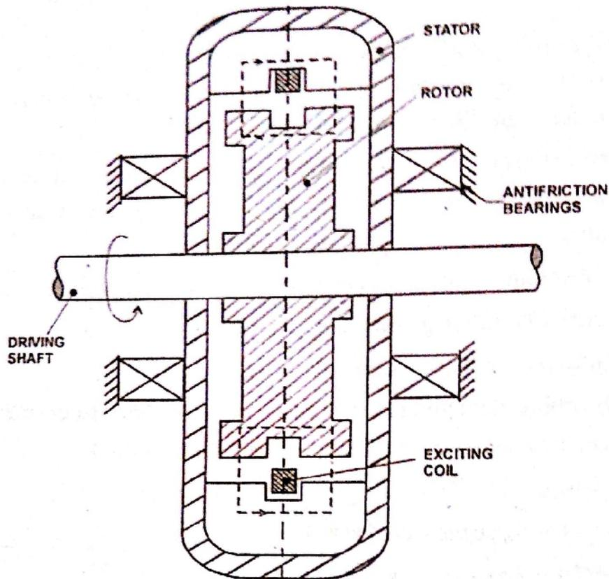
Figure 12.3: Eddy current dynamometer
