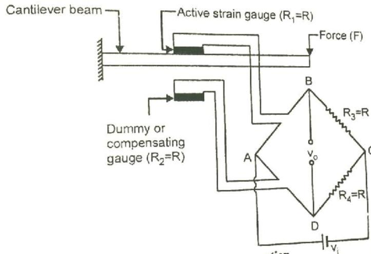
*Use of dummy gauge for temperature compensation.*
