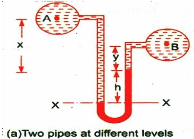
Fig (a) Let two points A and B are at a different level and also contain liquids of different Sp. gr. These points are connected to the U-tube differential manometer.
