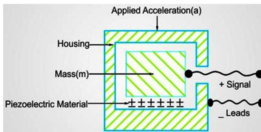
Compared to other type of accelerometers, piezoelectric accelerometers offer unique advantages
