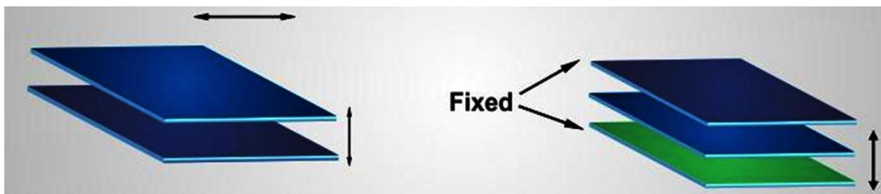
In these accelerometers, a diaphragm acting as a mass moves in the presence of acceleration. The diaphragm is sandwiched between the two fixed plates creating two capacitors; each with an individual fixed plate and each sharing the diaphragm as a movable plate. Movement of the diaphragm causes a capacitance shift by altering the distance between two parallel plates, the diaphragm itself being one of the plates.
