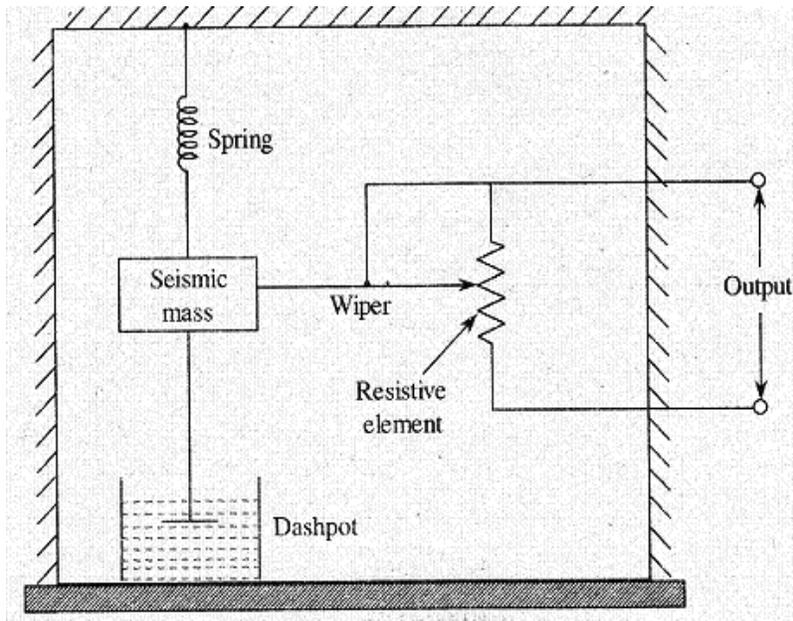
fig 9.1 Potentiometric accelerometer
