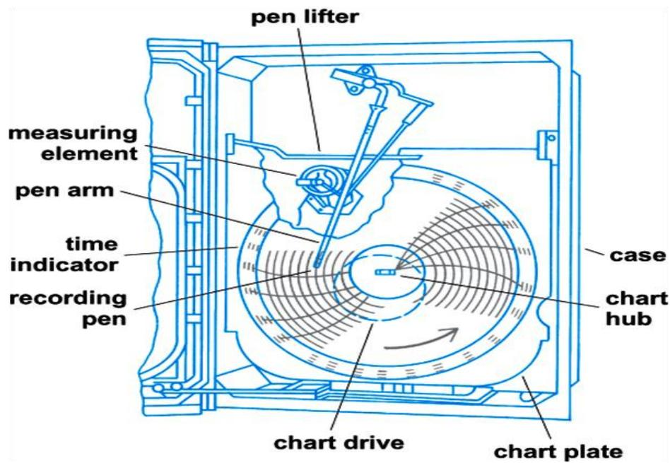
The complete instrument is often named a “-graph,” for example, a barograph for recording barometric pressure data, a tachograph for recording the time and velocity that a vehicle is in motion, or a seismograph for recording seismic waves.
