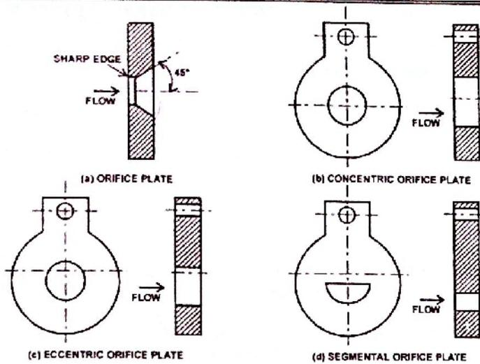
Figure 21.1: Shape of orifice plate
