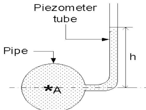
The tube extends vertically upward to such a height that liquid can freely rise in it without overflowing. The pressure at any point in the liquid is indicated by the height of the liquid in the tube above that point.
