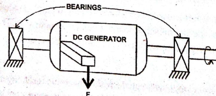
Figure 12.4: DC cradled dynamometer
