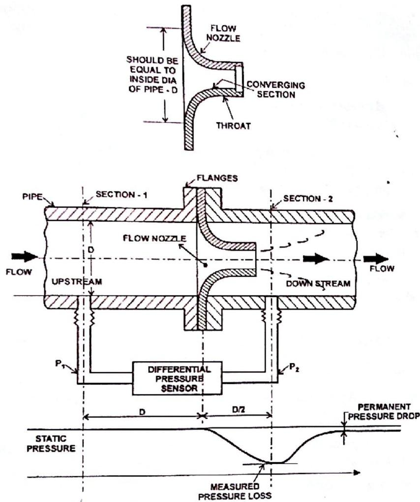
Figure 21.3: Flow nozzle arrangement
