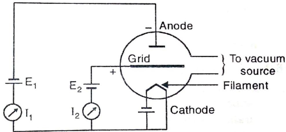
***Hot-filament ionization gauge.***
