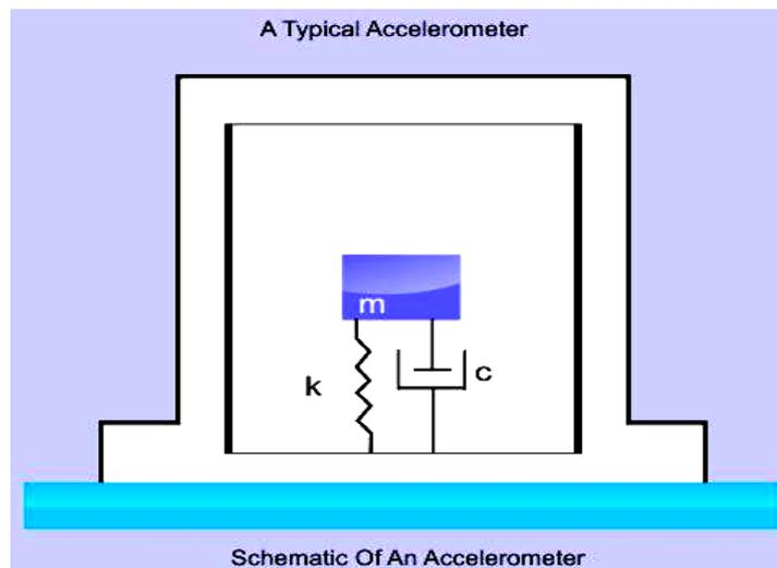
When the system is subjected to linear acceleration, a force (= mass \* acceleration) acts on the proof-mass. This causes it to deflect; the deflection is sensed by a suitable means and is converted into an equivalent electrical signal.
