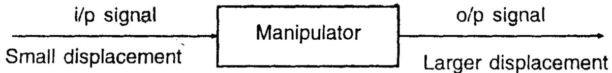
Therefore, output signal = input signal  $\times$  some constant
