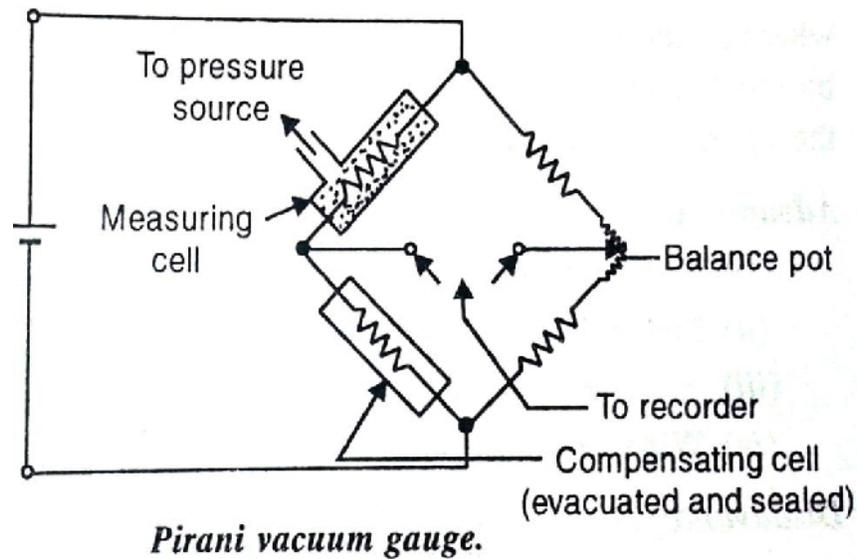
As the surrounding pressure changes, the filament temperature and hence its resistance also changes. A compensating cell is also employed to minimize variation caused by ambient temperature changes. The resistance change of the filament in the measuring cell is measured by the use of a resistance bridge which is calibrated in terms of pressure.
