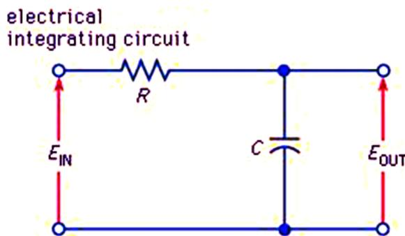
For time-varying input, if the resistance  $R$  shown in the schematic diagram is very large compared with the capacitive reactance  $X_C$  of the capacitor  $C$ , the current will be almost in phase with the input
