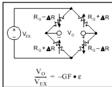
**Figure 7. Full-Bridge Circuit**
