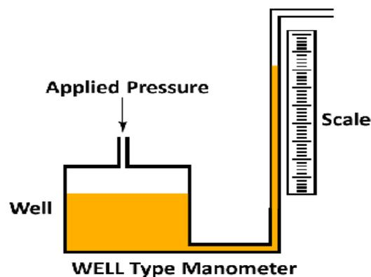
Thus, the well manometer provides an easier means of reading pressure. No longer does one have to measure the difference of height between two liquid columns, only the height of a single column.
