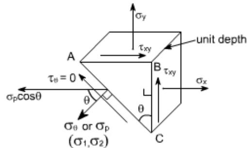
Consider once again the equilibrium of a triangular block of material of unit depth, Assuming AC to be a principal plane on which principal stresses  $\sigma_p$  acts, and the shear stress is zero.
