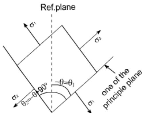
If we just want to measure the angles from the reference plane, than rotate this block through  $180^\circ$  so as to have the following appearance.
