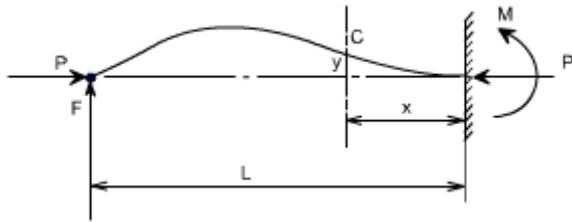
In order to maintain the pin-joint on the horizontal axis of the unloaded strut, it is necessary in this case to introduce a vertical load  $F$  at the pin. The moment of  $F$  about the built in end then balances the fixing moment.
