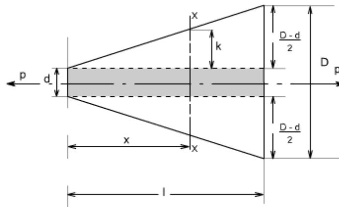
In order to compute the value of diameter of a bar at a chosen location let us determine the value of dimension  $k$ , from similar triangles
