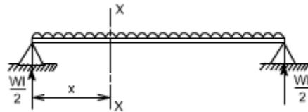
$$\begin{aligned} \text{S.F.}|_{x-x} &= w\left(\frac{l}{2}\right) - w \cdot x \\ \text{B.M.}|_{x-x} &= w\left(\frac{l}{2}\right) \cdot x - w \cdot x \cdot \left(\frac{x}{2}\right) \\ &= \frac{wl \cdot x}{2} - \frac{wx^2}{2} \end{aligned}$$
