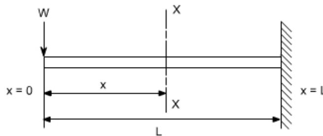
In order to solve this problem, consider any X-section X-X located at a distance x from the left end or the reference, and write down the expressions for the shear force and the bending moment
