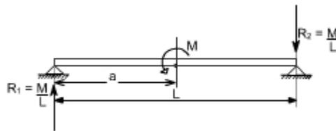
To deal with couples, only thing to remember is that within the pointed brackets we have to take some quantity and this should be raised to the power zero. i.e.  $M \langle x - a \rangle^0$ . We have taken the power 0 (zero) ' because ultimately the term  $M \langle x - a \rangle^0$  should have the moment units. Thus with integration the quantity  $\langle x - a \rangle^0$  becomes either  $\langle x - a \rangle^1$  or  $\langle x - a \rangle^2$
