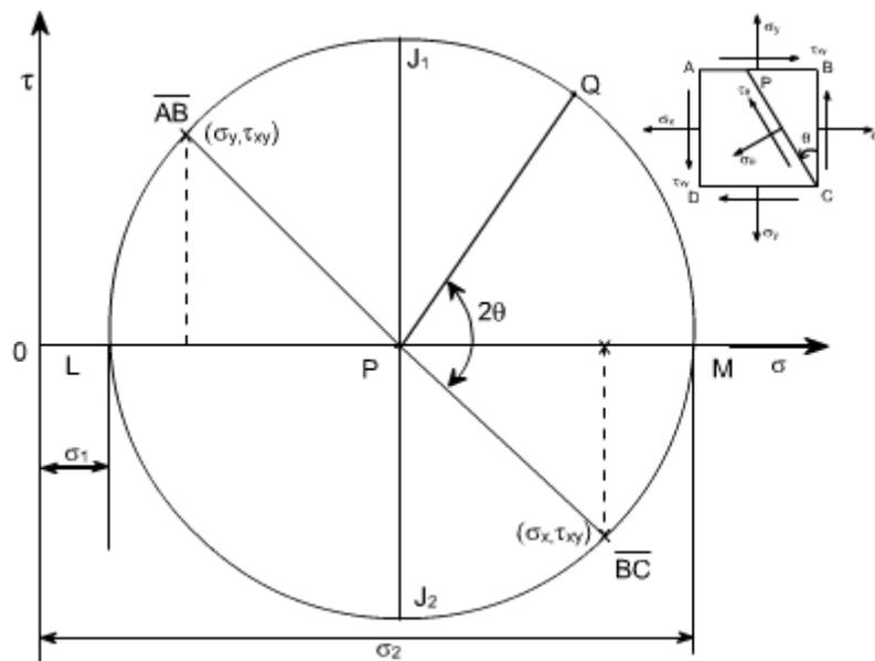
As we know that the circle represents all possible states of normal and shear stress on any plane through a stresses point in a material. Further we have seen that the co-ordinates of the point 'Q' are seen to be the same as those derived from
