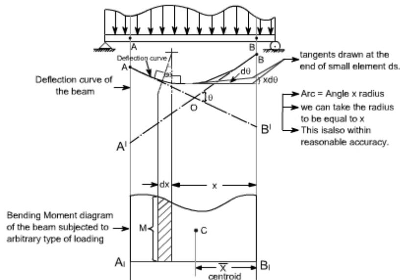
Refer to the figure shown above consider AB to be any portion of the elastic line of the loaded beam and A<sub>1</sub>B<sub>1</sub> is its corresponding bending moment diagram.
