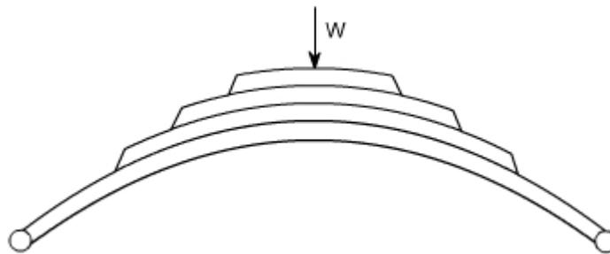
These type of springs are used in the automobile suspension system.
