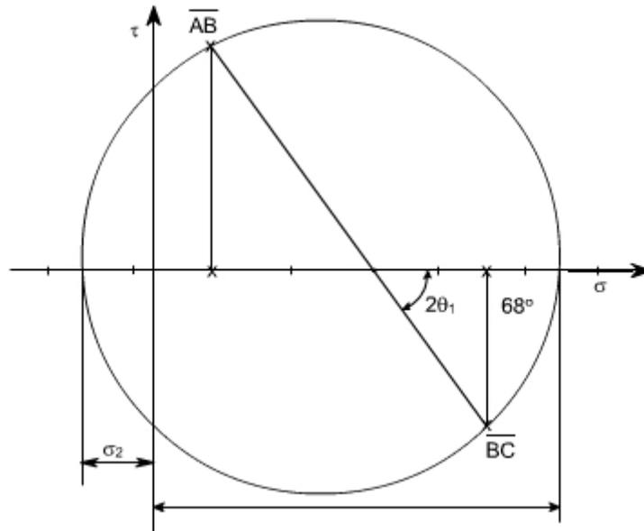
Taking the measurements from the Mohr's stress circle, the various quantities computed are
