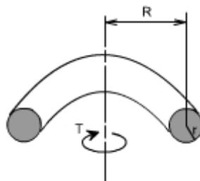
In this case the material of the spring is subjected to pure bending which tends to reduce Radius R of the coils. In this case the bending moment is constant throughout the spring and is equal to the applied axial Torque T. The stresses i.e. maximum
