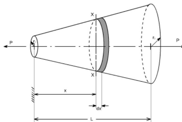
consider the above figure let  $r_1$  be the radius at the smaller end. Then at a X crossection XX located at a distance  $x$  from the smaller end, the value of radius is equal to
