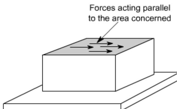
The resulting force intensities are known as shear stresses, the mean shear stress being equal to
