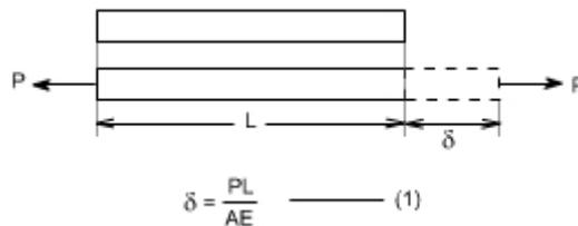
Suppose the bar is loaded at one or more intermediate positions, then equation (1) can be readily adapted to handle this situation, i.e. we can determine the axial force in each part of the bar i.e. parts AB, BC, CD, and calculate the elongation or shortening of each part separately, finally, these changes in lengths can be added algebraically to obtain the total change in length of the entire bar.
