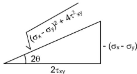
Because of root the difference in sign convention arises from the point of view of locating the planes on which shear stress act. From physical point of view these sign have no meaning.
