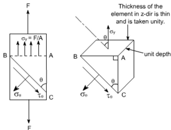
The stress acting at a point is represented by the stresses acting on the faces of the element enclosing the point. The stresses change with the inclination of the planes passing through that point i.e. the stress on the faces of the element vary as the angular position of the element changes. Let the block be of unit depth now considering the equilibrium of forces on the triangle portion ABC. Resolving forces perpendicular to BC, gives
