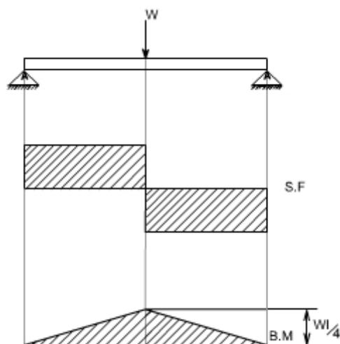
It may be observed that at the point of application of load there is an abrupt change in the shear force, at this point the B.M is maximum.
