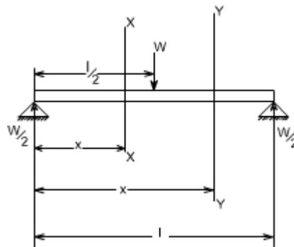
.So the shear force at any X-section would be  $= W/2$  [Which is constant upto  $x < l/2$ ]
