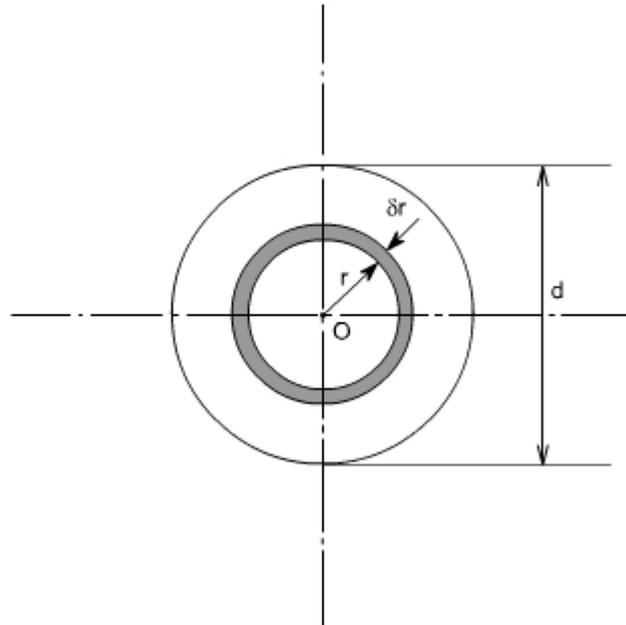
Consider any circular strip of thickness  $\delta r$  located at a radius 'r'.
