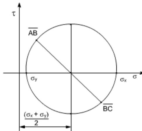
(4) As already defined the principal planes are the planes on which the shear components are zero.
