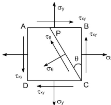
As per the double subscript notation the shear stress on the face BC should be notified as  $\tau_{yx}$ , however, we have already seen that for a pair of shear stresses there is a set of complementary shear stresses generated such that  $\tau_{yx} = \tau_{xy}$
