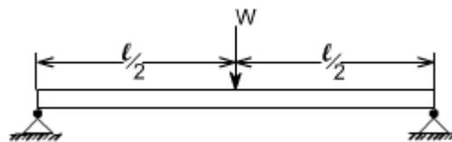
By symmetry the reactions at the two supports would be  $W/2$  and  $W/2$ . now consider any section X-X from the left end then, the beam is under the action of following forces.
