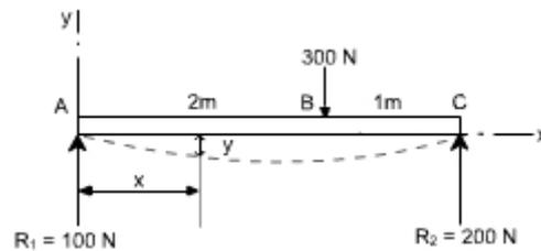
**Solution :** writing the general moment equation for the last portion BC of the loaded beam,
