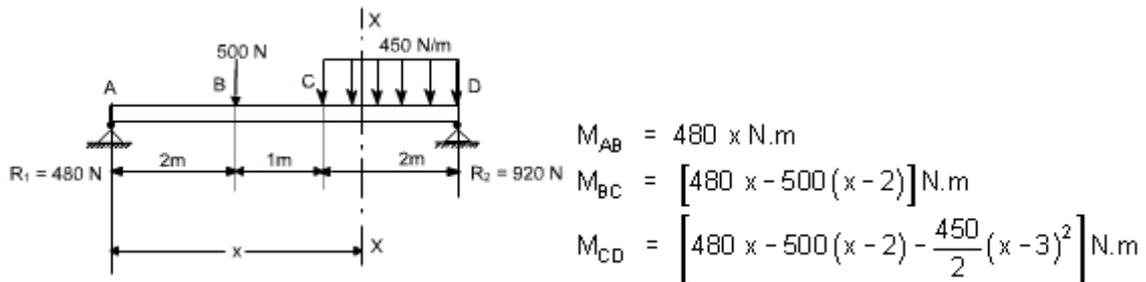
It may be observed that the equation for  $M_{CD}$  will also be valid for both  $M_{AB}$  and  $M_{BC}$  provided that the terms  $(x - 2)$  and  $(x - 3)^2$  are neglected for values of  $x$  less than 2 m and 3 m, respectively. In other words, the terms  $(x - 2)$  and  $(x - 3)^2$  are nonexistent for values of  $x$  for which the terms in parentheses are negative.
