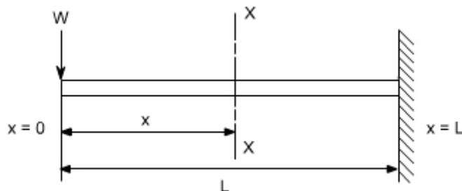
In order to solve this problem, consider any X-section X-X located at a distance  $x$  from the left end or the reference, and write down the expressions for the shear force and the bending moment
