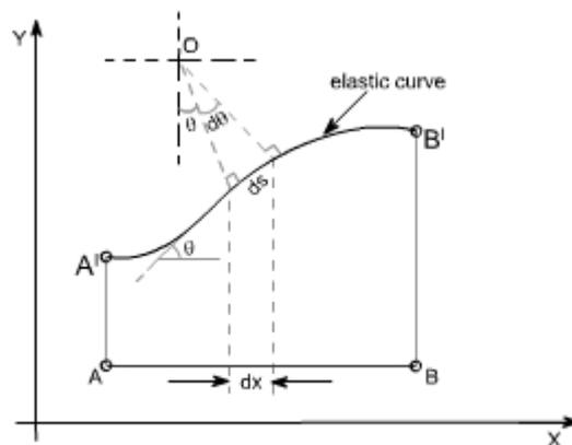
It may be noted that \$d\theta\$ is an angle subtended by an arc element \$ds\$ and \$M\$ is the bending moment to which this element is subjected.
