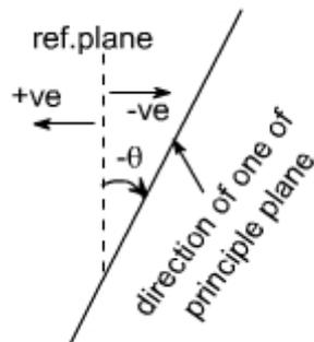
Therefore the direction of other principal planes would be  $\{\theta + 90\}$  since the angle  $\theta$  is always less in magnitude than  $90$  hence the quantity  $(\theta + 90)$  would be positive therefore the Inclination of other plane with reference plane would be positive therefore if just complete the Block. It would appear as
