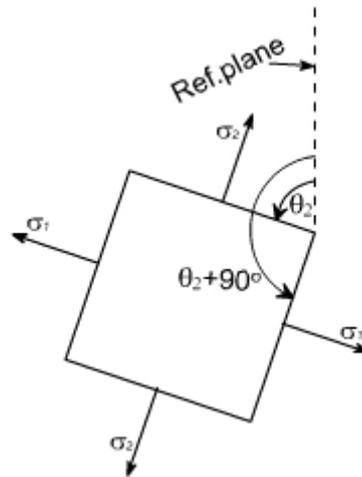
So whenever one of the angles comes negative to get the positive value, first Add  $90^\circ$  to the value and again add  $90^\circ$  as in this case  $\theta_2 = 23^\circ 74'$  so  $\theta_1 = 23^\circ 74' + 90^\circ = 66^\circ 26'$ . Again adding  $90^\circ$  also gives the direction of other principle planes
