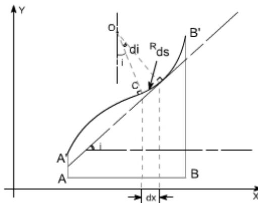
Consider a beam AB which is initially straight and horizontal when unloaded. If under the action of loads the beam deflects to a position A'B' under load or in fact we say that the axis of the beam bends to a shape A'B'. It is customary to call A'B' the curved axis of the beam as the elastic line or deflection curve.
