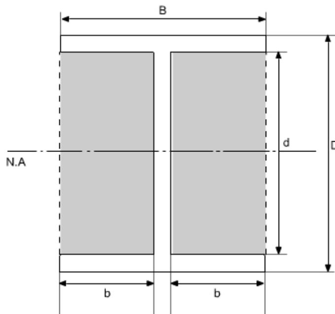
$$I_{N.A.} = I_{\text{of dotted rectangle}} - I_{\text{of shaded portion}}$$
