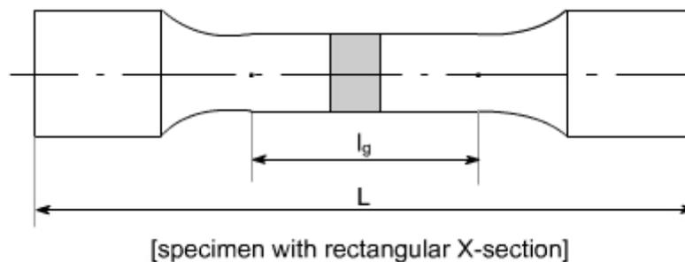
$l_g$  = gauge length i.e. length of the specimen on which we want to determine the mechanical properties. The uniaxial tension test is carried out on tensile testing machine and the following steps are performed to conduct this test.
