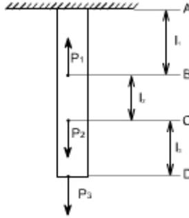
When either the axial force or the cross – sectional area varies continuously along the axis of the bar, then equation (1) is no longer suitable. Instead, the elongation can be found by considering a differential element of a bar and then the equation (1) becomes
