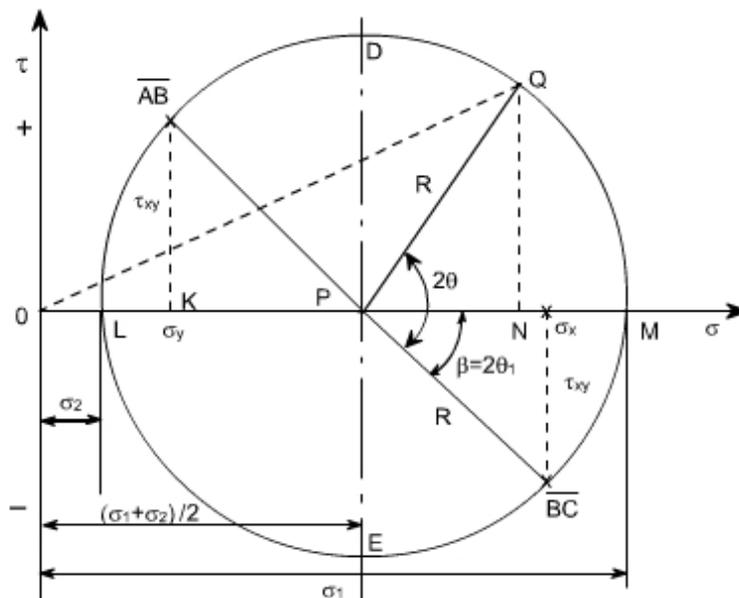
Consider any point Q on the circumference of the circle, such that PQ makes an angle  $2\alpha$  with BC, and drop a perpendicular from Q to meet the s axis at N. Then OQ represents the resultant stress on the plane an angle  $\alpha$  to BC. Here we have assumed that  $\sigma_x < \sigma_y$
