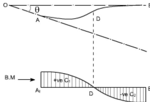
Then, adequate precaution must be exercised in using the above theorem. In such a case B. M diagram gets divide into two portions +ve and -ve portions with centroids  $C_1$  and  $C_2$ . Then to find an angle  $\theta$  between the tangents at the points A and B
