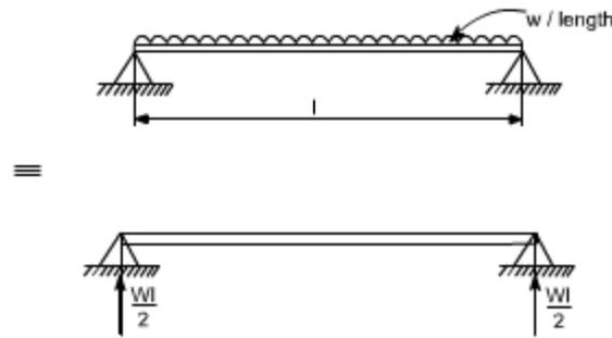
In order to write down the expression for bending moment consider any cross-section at distance of  $x$  metre from left end support.
