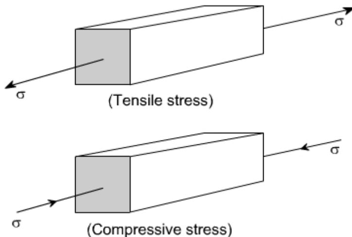
**Bearing Stress:** When one object presses against another, it is referred to a bearing stress ( They are in fact the compressive stresses ).
