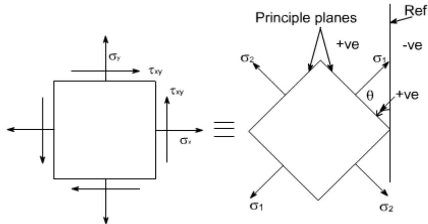
Let us recall that for the case of a material subjected to direct stresses the value of maximum shear stresses
