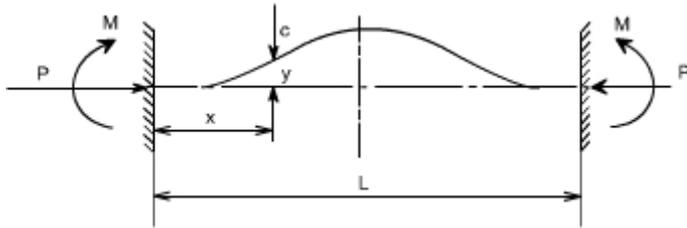
Due to the fixed end supports bending moment would also appears at the supports, since this is the property of the support.
