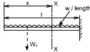
Here the cantilever beam is subjected to a uniformly distributed load whose intensity is given  $w / \text{length}$ .
