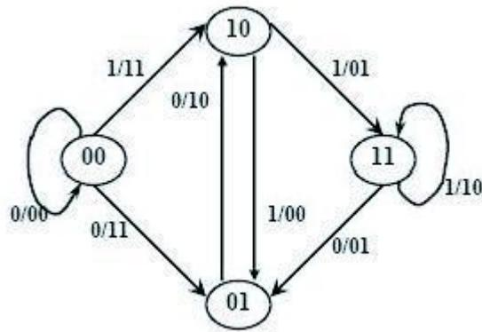
**Figure 4.6: State diagram representation of a convolutional encoder**
