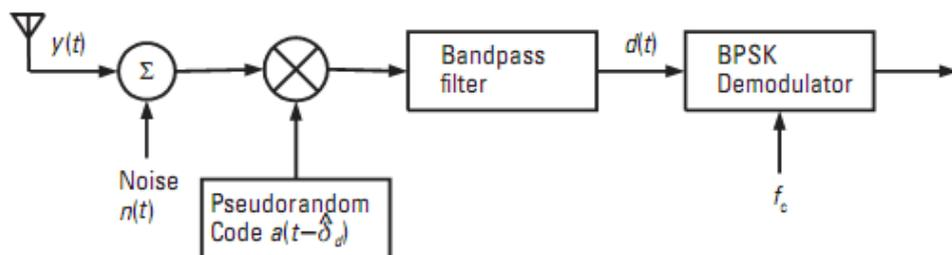
**Figure 4.3 Block diagram of a DS-SS Receiver**
