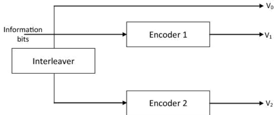
Figure 4.7: Block diagram of a turbo encoder
