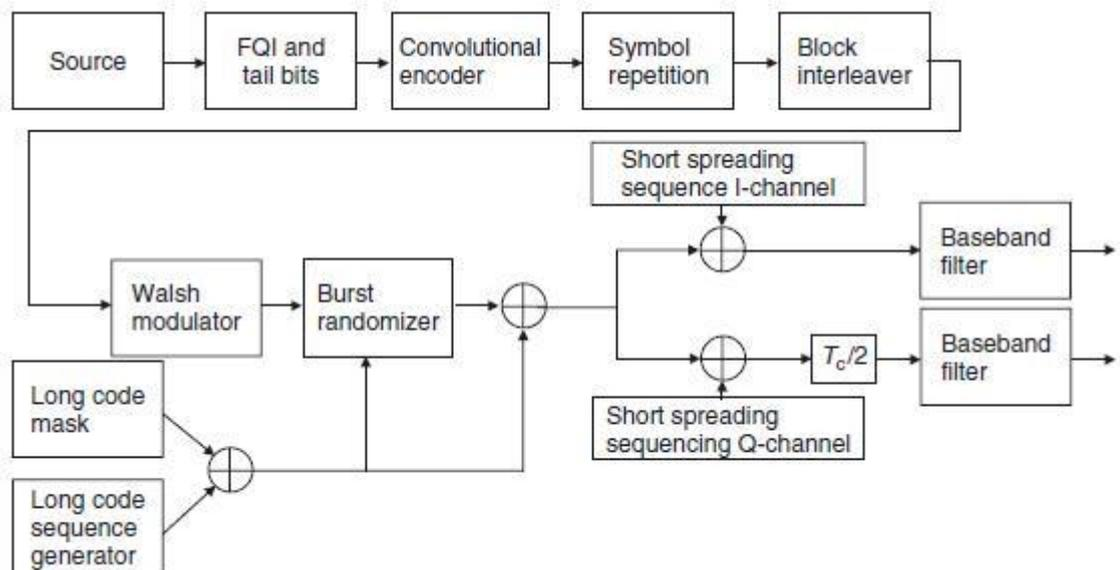
Figure 4.7: Block diagram of an IS-95 mobile station transmitter
