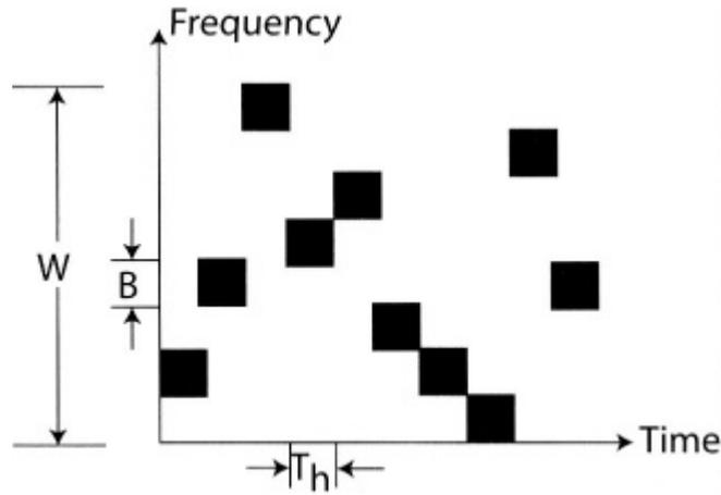
**Figure 4.4: Frequency Hopping Pattern of a FHSS system**
