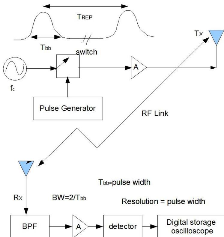
Figure 5.4: Direct RF pulsed channel IR measurement.
