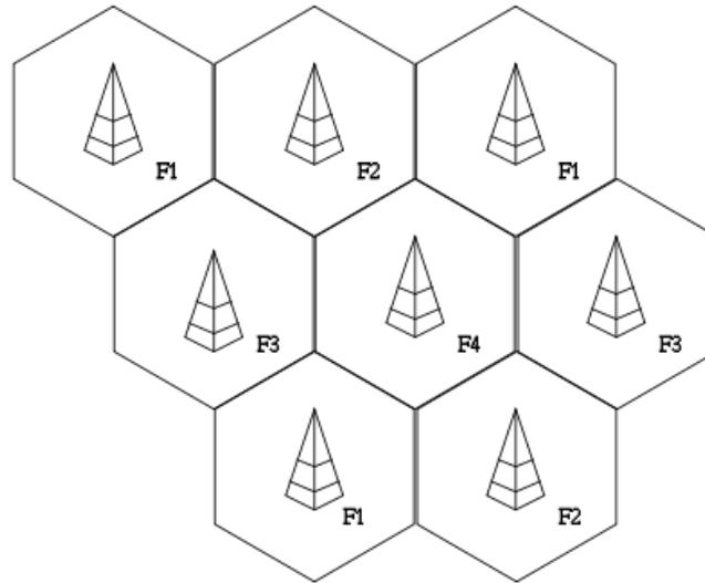
**Figure 1.5: Frequency reuse concept and cell splitting**
