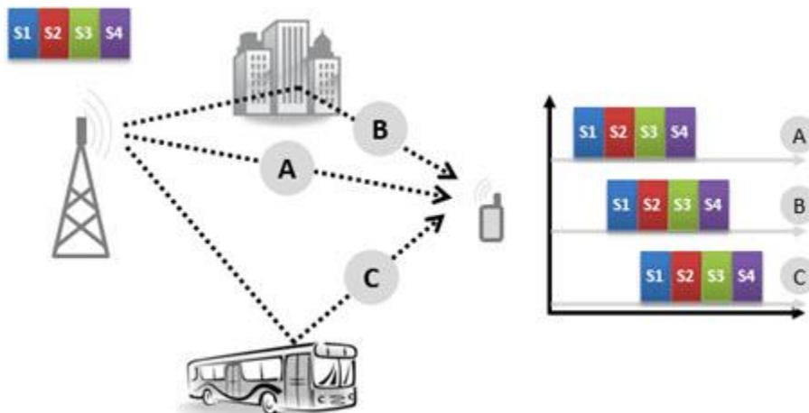
Although the "Multipath" bring positive benefits, "Multipath" and "Delay Spread" also end up causing interference inter symbols.
