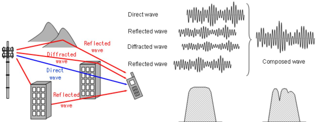
**Figure 1.15: Fading impact on signal amplitudes.**
