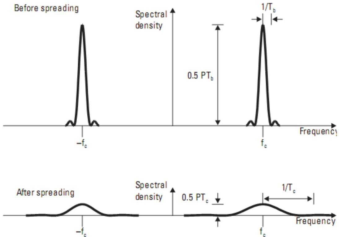
**Figure 4.2 Signal spectrum of DS-SS modulation before and after spreading**
