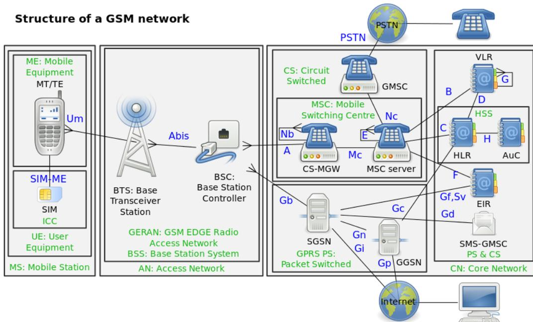
**Figure 1.2 : Structure of GSM Network**
