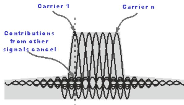
Figure 4.8:OFDM Spectrum
