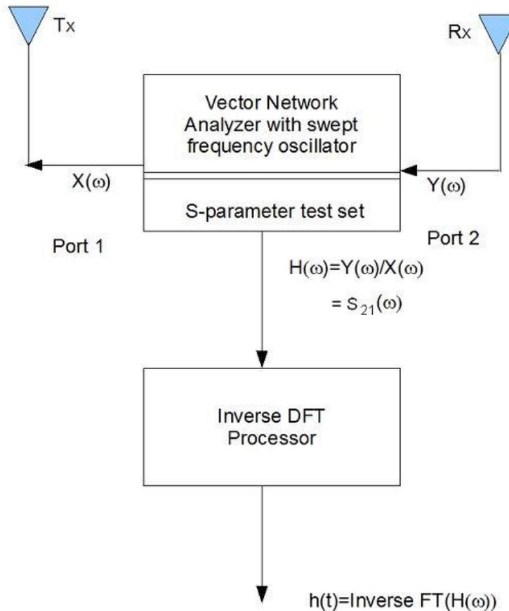
Frequency domain channel IR measurement
