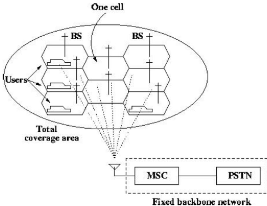
Figure 4.10 :Basic cellular structure
