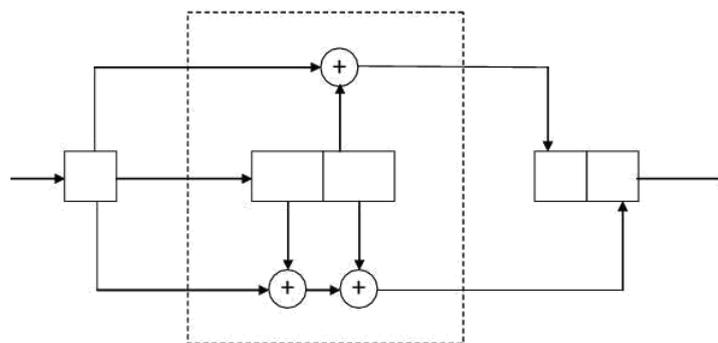
**Figure 4.5: A convolutional encoder with  $n=2$  and  $k=1$ .**
