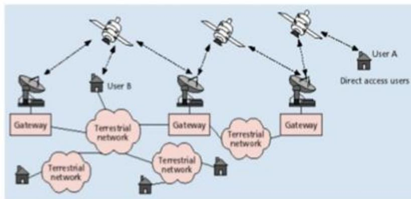
**Figure 1.10: Call establishment between user A and user B**
