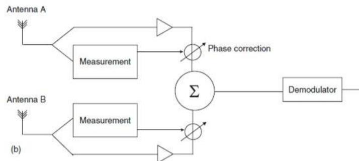
Figure 3.2 :Equal Gain Combining
