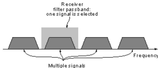
Figure 4.7 :Traditional view of receiving signals carrying modulation
