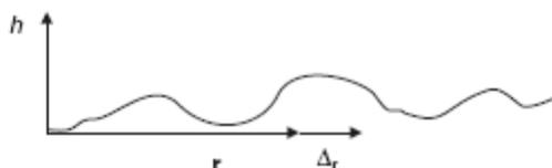
Figure 4.14 Geometry for perturbation theory of rough scattering.
