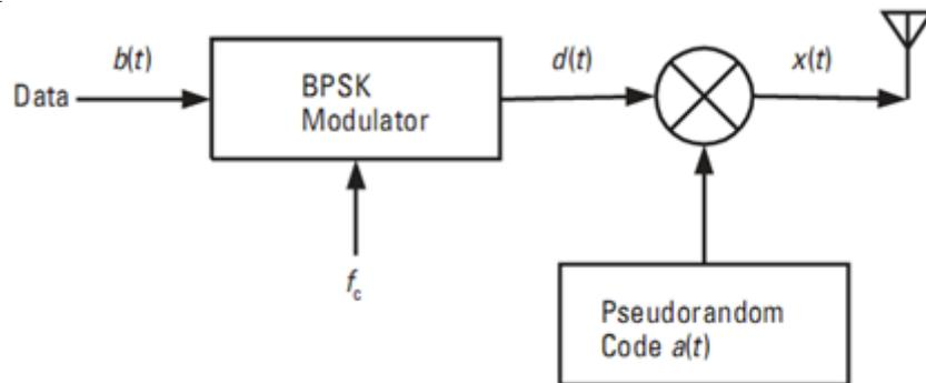
**Figure 4.1 Block diagram of DS-SS Transmitter**
